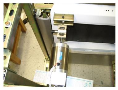
3-10: Mounted Load Cell and Actuator
