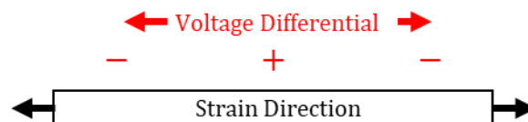
Figure 4.2: Strain Develops in the same direction as the Voltage Differential in a d33 MFC
