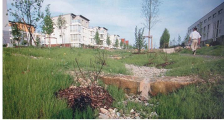
fig. 1l: Stormwater used as both amenity park/walkway and water filtration (Reed, P.)
