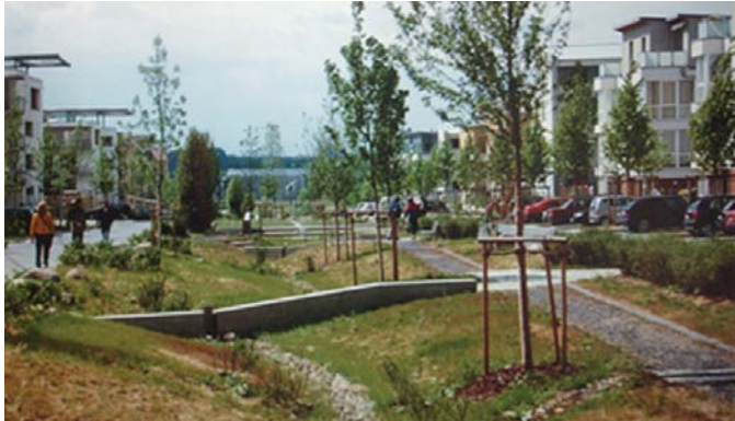
fig. 1l: Stormwater used as both amenity park/walkway and water filtration (Reed, P.)
