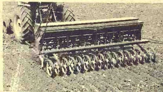
International 150 shovel press drills are offered in 8 sizes, 8, 10, 12, or 14-inch spacings.
