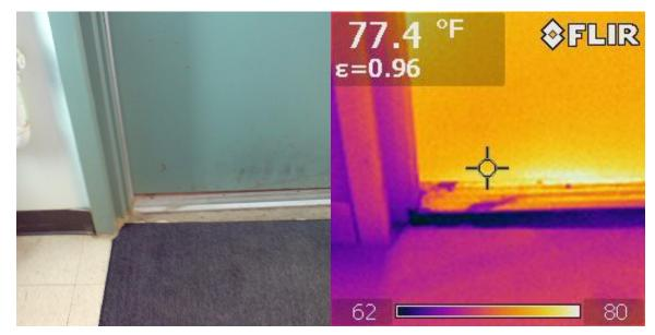
Figure 7.36 Infiltration Detection—Exterior Door
