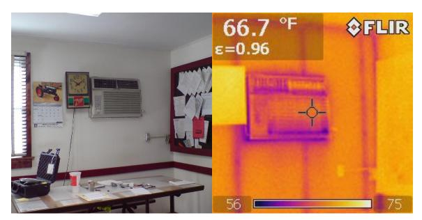
Figure 7.54 Infiltration Detection—Wall Penetration and Construction
