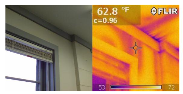
Figure 7.23 Infiltration Detection—Wall and Ceiling Seam
