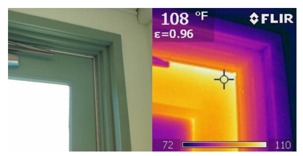
Figure 7.37 Infiltration Detection—Exterior Door
