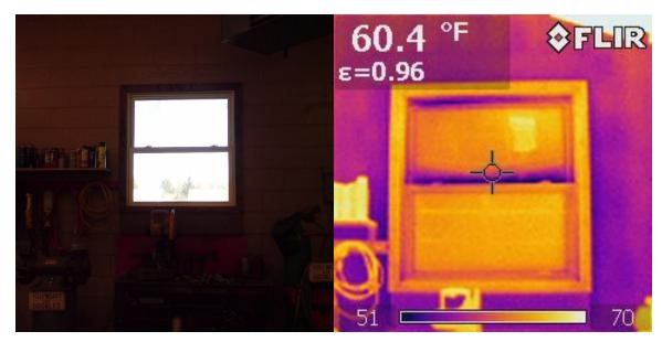
Figure 7.55 Infiltration Detection—Bay Window
