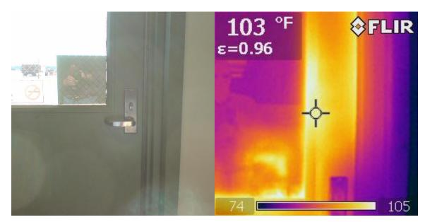
Figure 7.40 Infiltration Detection—Exterior Door
