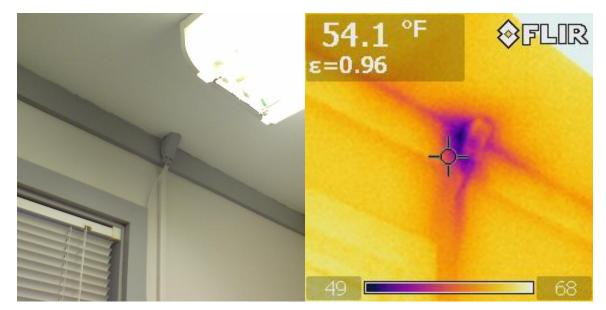
**Figure 7.24 Infiltration Detection—Ceiling Penetration**
