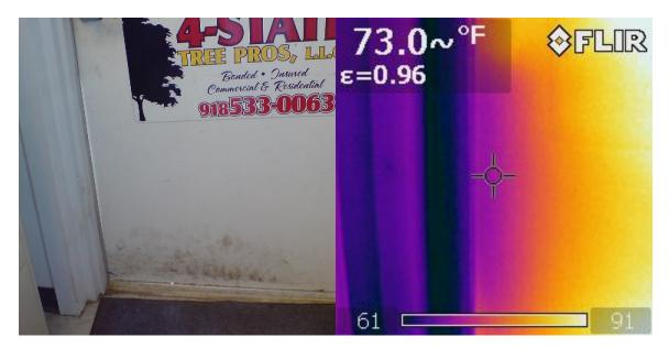
Figure 7.49 Infiltration Detection—Exterior Door
