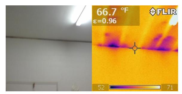
Figure 7.27 Infiltration Detection—Wall and Ceiling Seam
