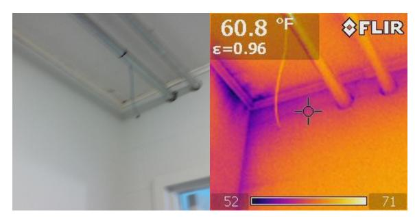
Figure 7.46 Infiltration Detection—Wall Penetrations and Seams
