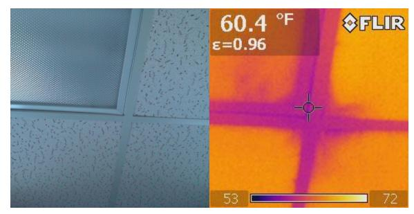
Figure 7.45 Infiltration Detection—Ceiling Grid Seams
