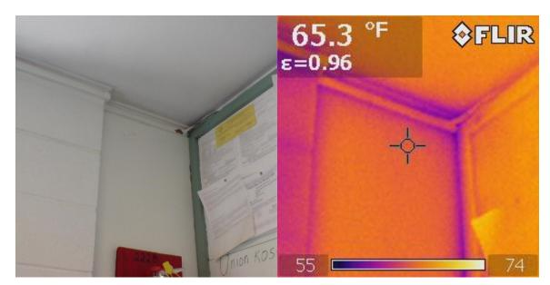
Figure 7.34 Infiltration Detection—Wall and Ceiling Seams
