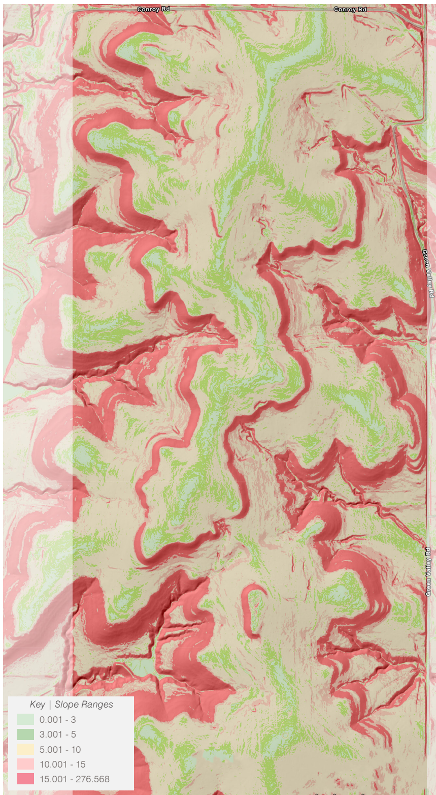
Figure 3.19. Developable slope area.
