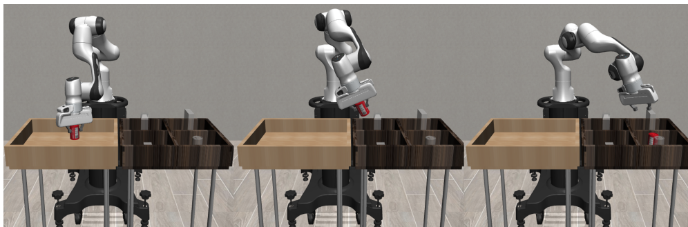
Figure 5.4: RoboSuite Pick-and-Place evaluation. The task requires grasping, transport, and placement under contact-rich manipulation dynamics.
