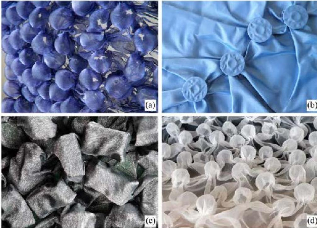
Figure 3. Binding over objects heat-set samples: (a) glass marbles bound closely in polyester/metallic organza, (b) metal bobbins in polyester satin lining, (c) plastic interlocking bricks in nylon organza, and (d) plastic beads in polyester organza. Photos by David Mayes and Sherry J. Haar.
