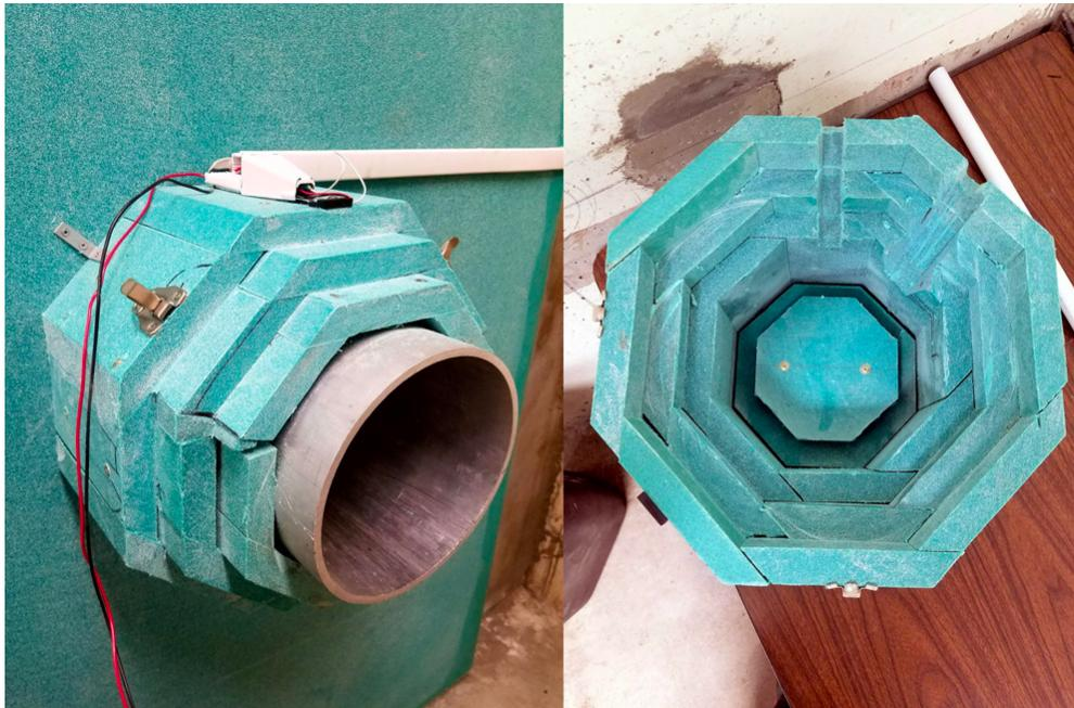
**Figure 5.13:** Removable shielding cap for borehole pipe
