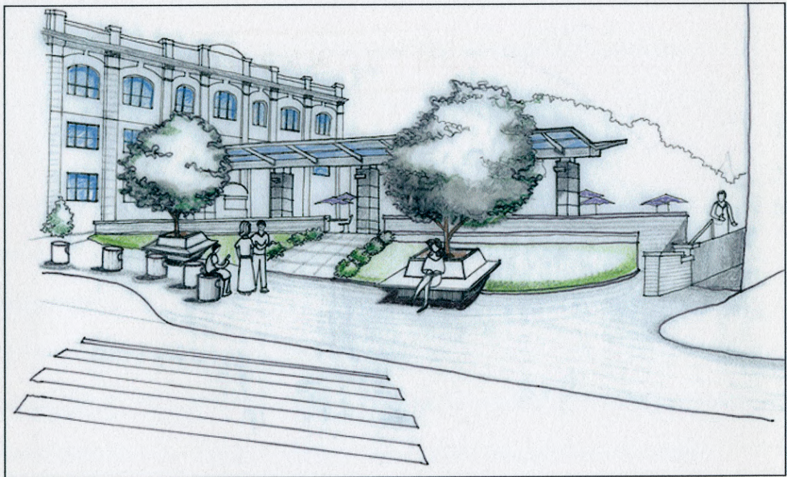
Figure 7.13: Two planters with backrests and seating bollards with lightings.
