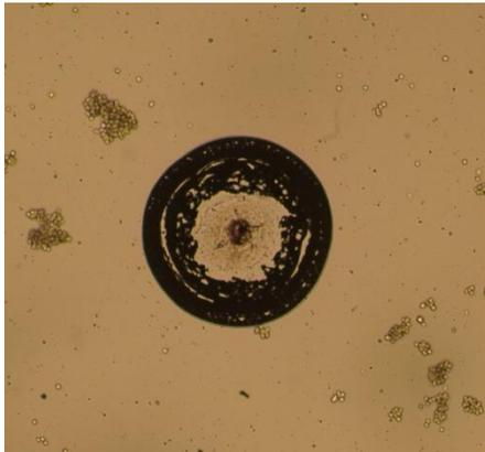
**Figure 4.2** A photograph of dielectric breakdown of a 40  $\mu\text{m}$  PDMS film. As dielectric breakdown occurs, high energy electrons burn a hole through the film and a visible electrical arc can be observed.
