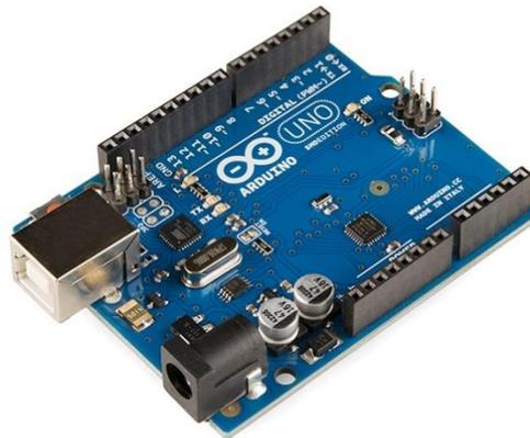
**Figure 1.9** A photograph of an Arduino UNO R3 microcontroller board.
