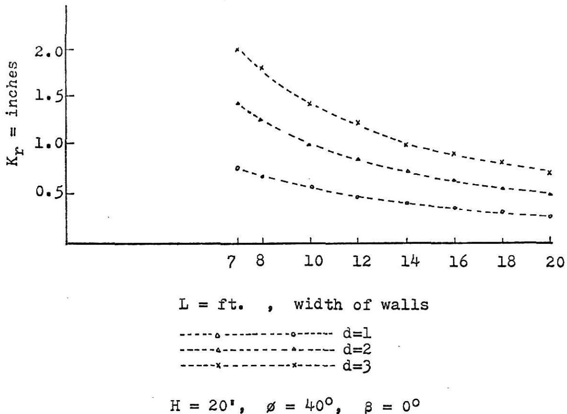
Fig. (14)  $K_r$  values with different separations of layers of the reinforcement, the wall height is 20 feet, and the internal friction angle of the soil  $\phi = 40^{\circ}$ , the Backfill  $\beta = 0^{\circ}$
