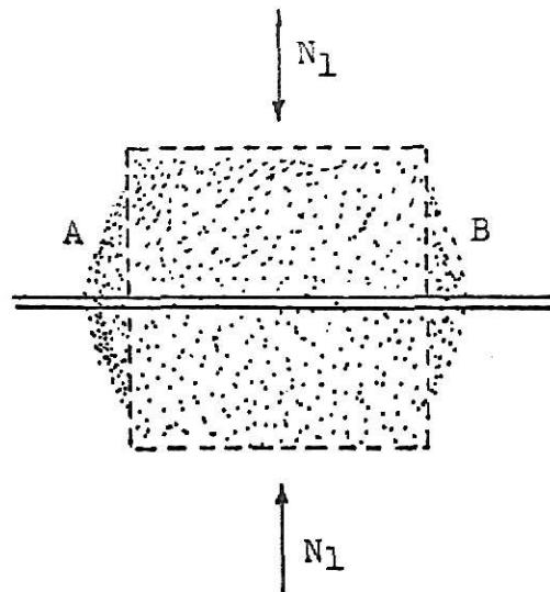
Fig. (8-a) A reinforcement is introduced horizontally into the cube of non-cohesive earth which is subjected to a vertical compressive force  $N_1$
