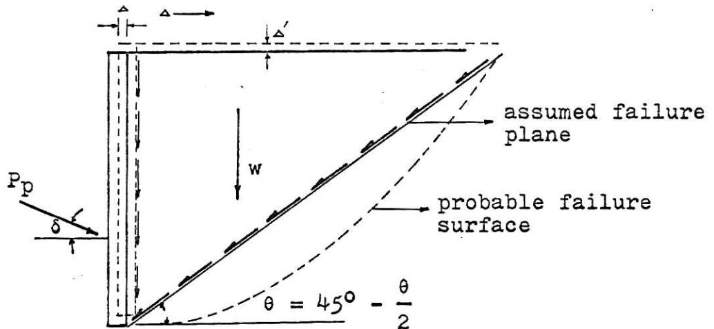
Fig. (2-b) Wall movement to develop passive pressure
