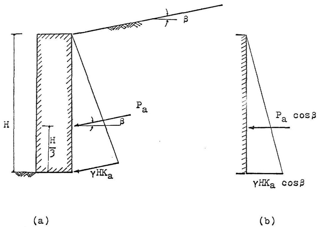
Fig. (9) (a) Active earth pressure diagram
