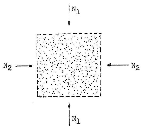
Fig. (7-a) A cube of non-cohesive earth is subjected to a compressive force  $N_1$  on its two faces, and  $N_2$  on its other axial two faces
