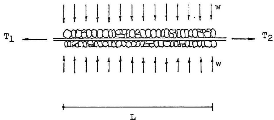
Fig. (5-a) A reinforcement is connected to the soil grains by tensions  $T_1$  and  $T_2$  and with the stress  $w$  normal to the reinforcement over a length  $L$
