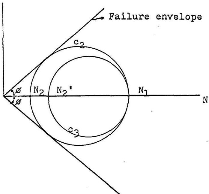
Fig. (7-b) Graphic representation of state of the stress at failure,  $c_2$ ,  $c_3$  represents the earth in elastic equilibrium
