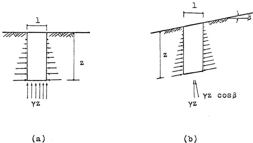
Fig. (1) (a) The vertical stress at depth  $z$
