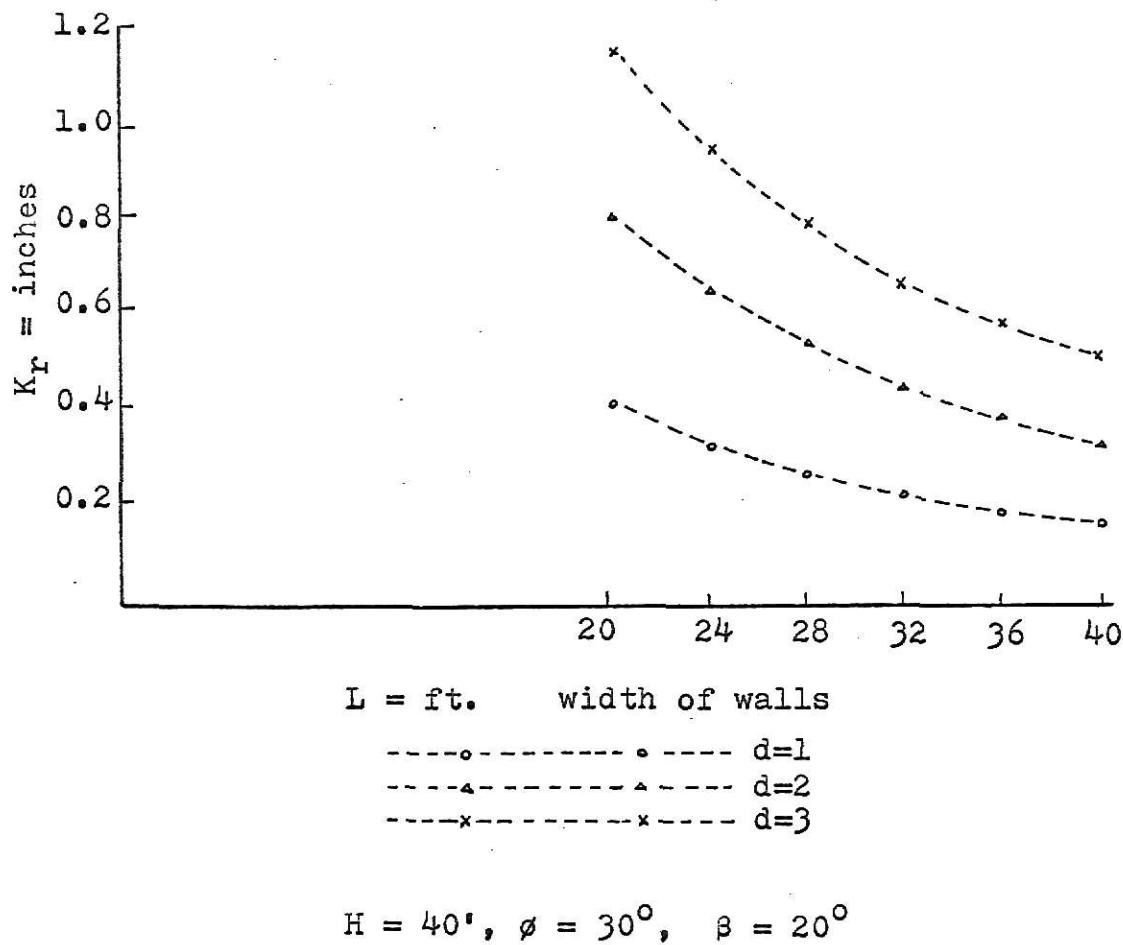
Fig. (16)  $K_r$  values with different separations of layers of the reinforcement, the wall height is 40feet, and the internal friction angle of the soil  $\phi = 30^{\circ}$ , the backfill  $\beta = 20^{\circ}$
