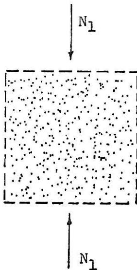
Fig. (6-a) A cube of non-cohesion earth
