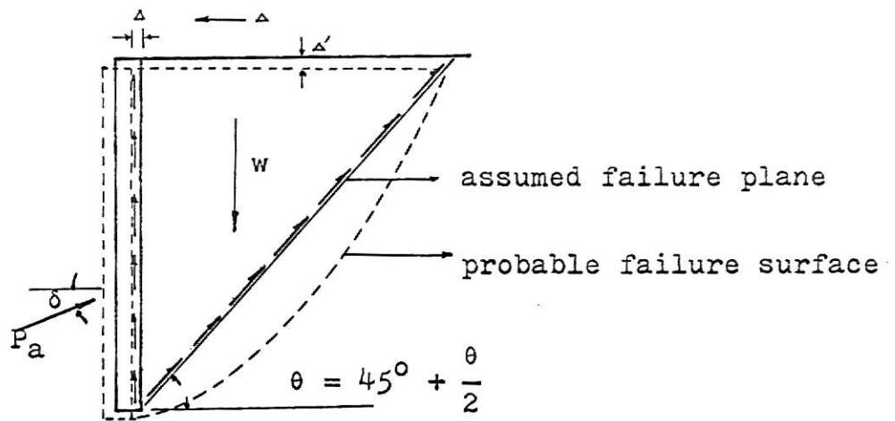
Fig. (2-a) Wall movement to develop active pressure
