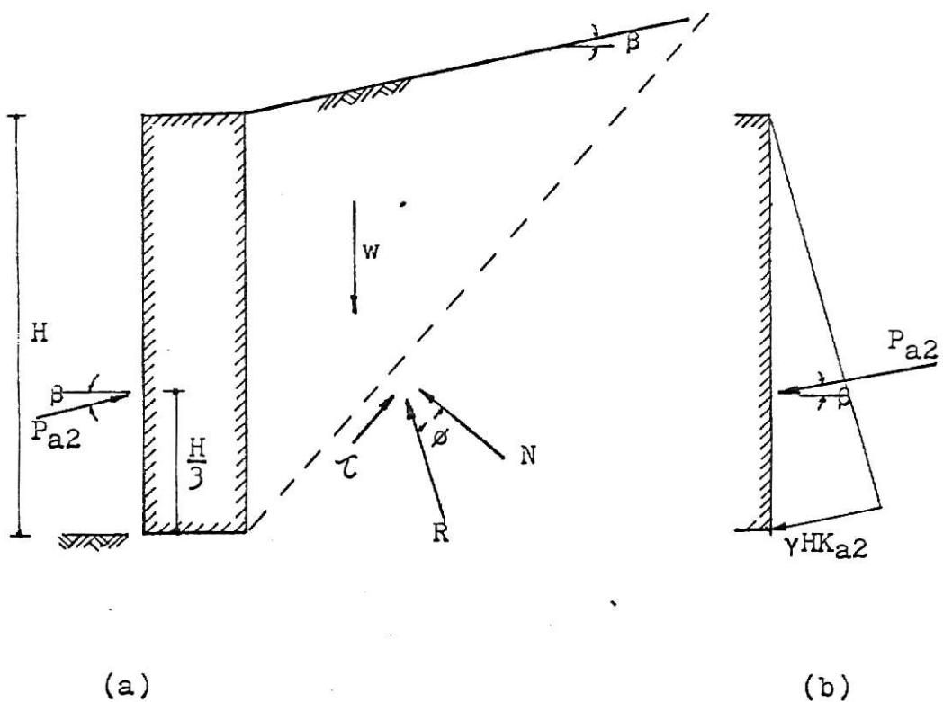
Fig. (4) (a) Failure wedge and acting forces
