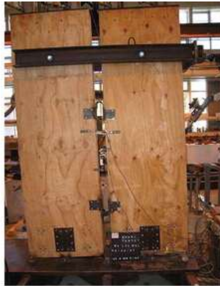
Figure 9. Coupled LVL Walls (Iqbal et al., 2015)
