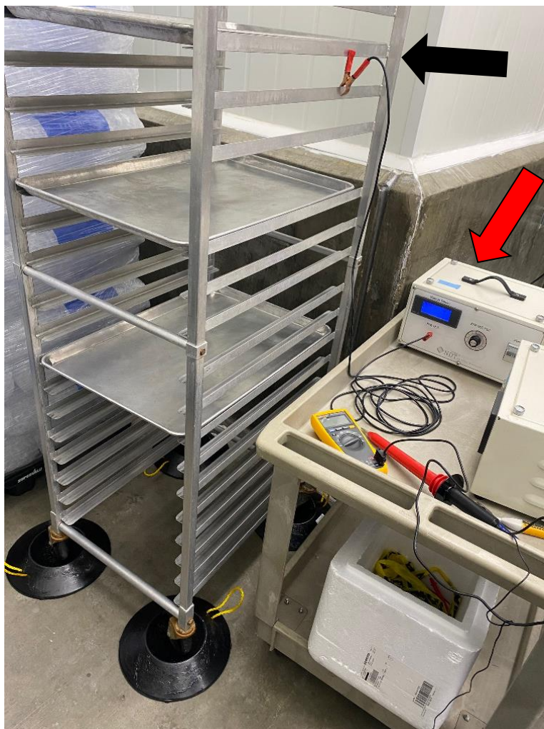
Figure 1. A representative image of the experiment setup using the electrostatic thawing system which consists of the electrostatic field (EF) generator (red arrow) and a stainless steel meat cart (black arrow).
