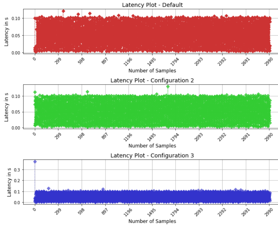
Figure 3.17. Latency Plots for liquid application and computer vision data collection in various configurations
