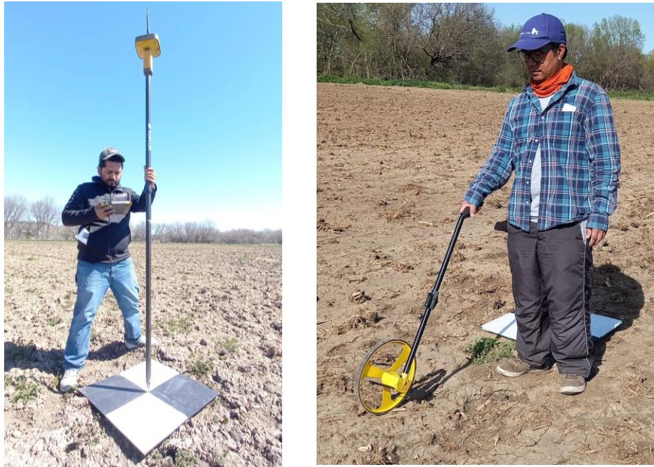
Figure 4.11. Recording geolocation of the GCP and measuring distance between each GCP
