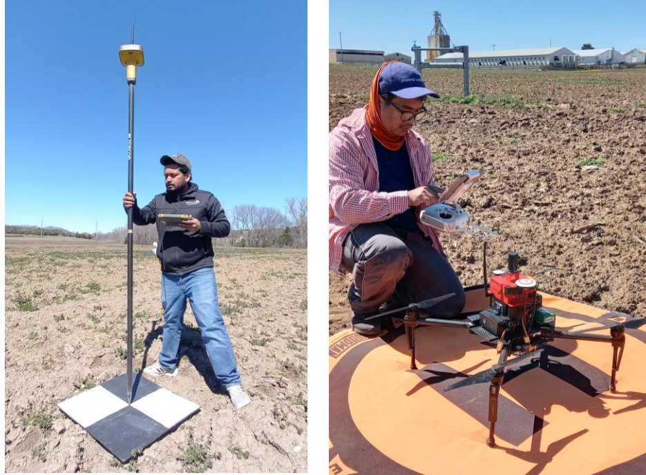
Figure 4.15. GCP co-ordinates collection and UAV flight setup
