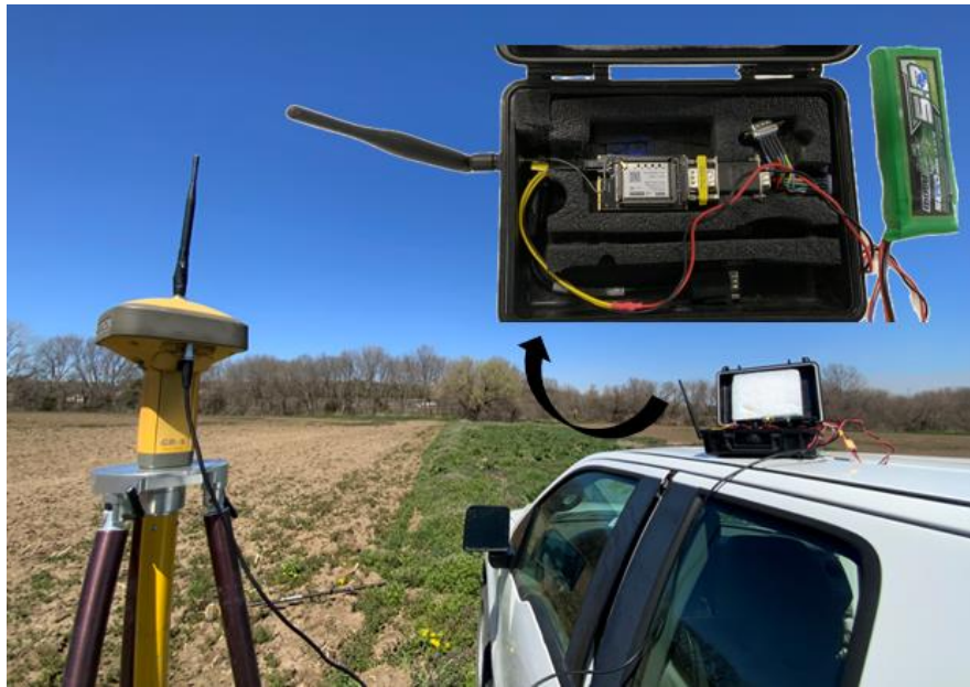
Figure 4.6. Base Station & Radio setup for RTK
