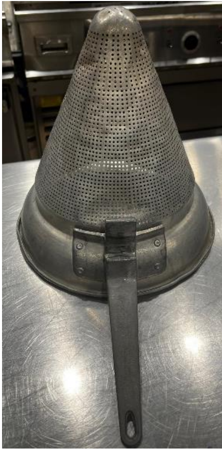
Figure 5.2 Conned shape strainer.
