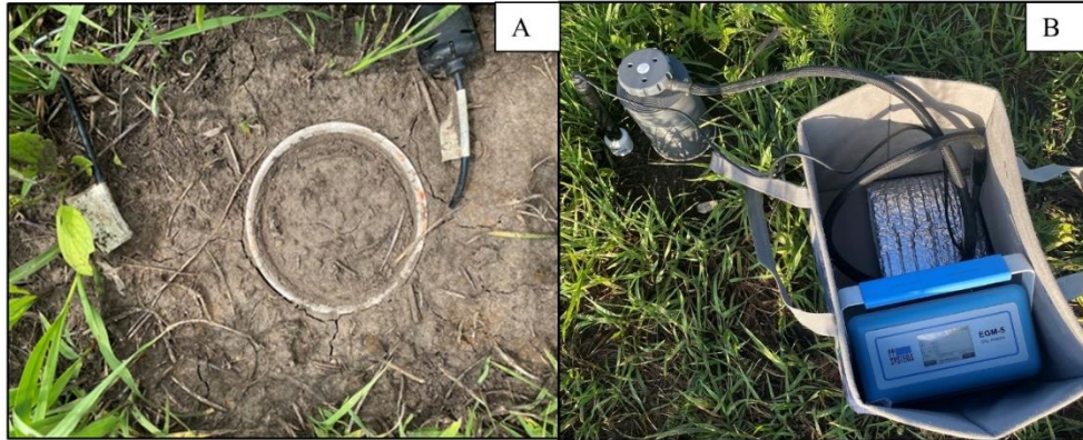
Figure 3-2: A) An installed instrumented PVC collar with sensors for measuring heterotrophic soil respiration, soil matric potential (model TEROS 21, Meter Group, Inc.), soil temperature (model TEROS 21, Meter Group, Inc.), and volumetric water content (model TEROS 10, Meter Group, Inc.) in a tallgrass prairie at Konza Prairie Biological Station near Manhattan, KS. Collars were maintained vegetation-free throughout the experimental period to assume CO 2 from collars is from heterotrophic soil respiration and B) measuring heterotrophic soil respiration from the installed instrumented PVC collars using a portable infrared CO 2 gas analyzer (model EGM-5, PP Systems, Inc.).
