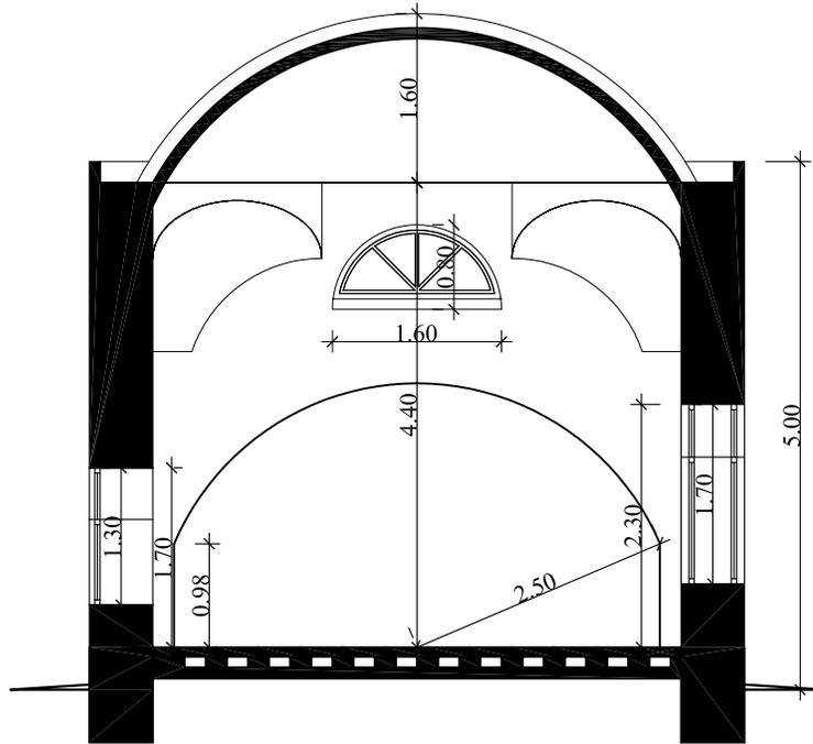
**FIG. 35** SINGLE CELL A-A SECTION
