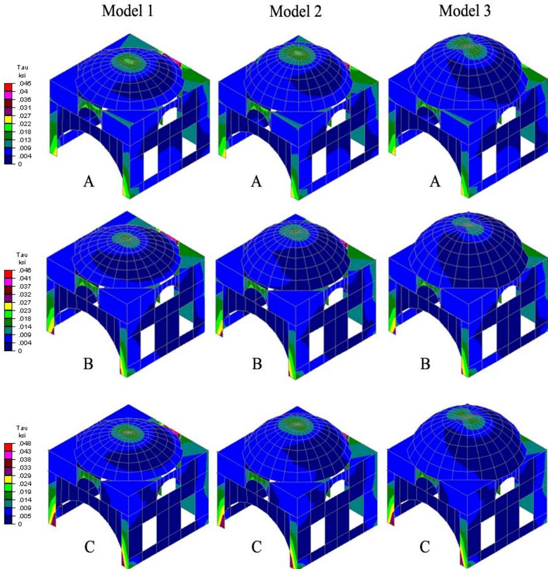
The shear stresses are six times less than the allowable stresses while on the other hand the traditional model was two times lower than the allowable stresses. None of the models show any structural problems. The model 1 roof gets a larger stress than the other two models, but the differences are structurally insignificant.
