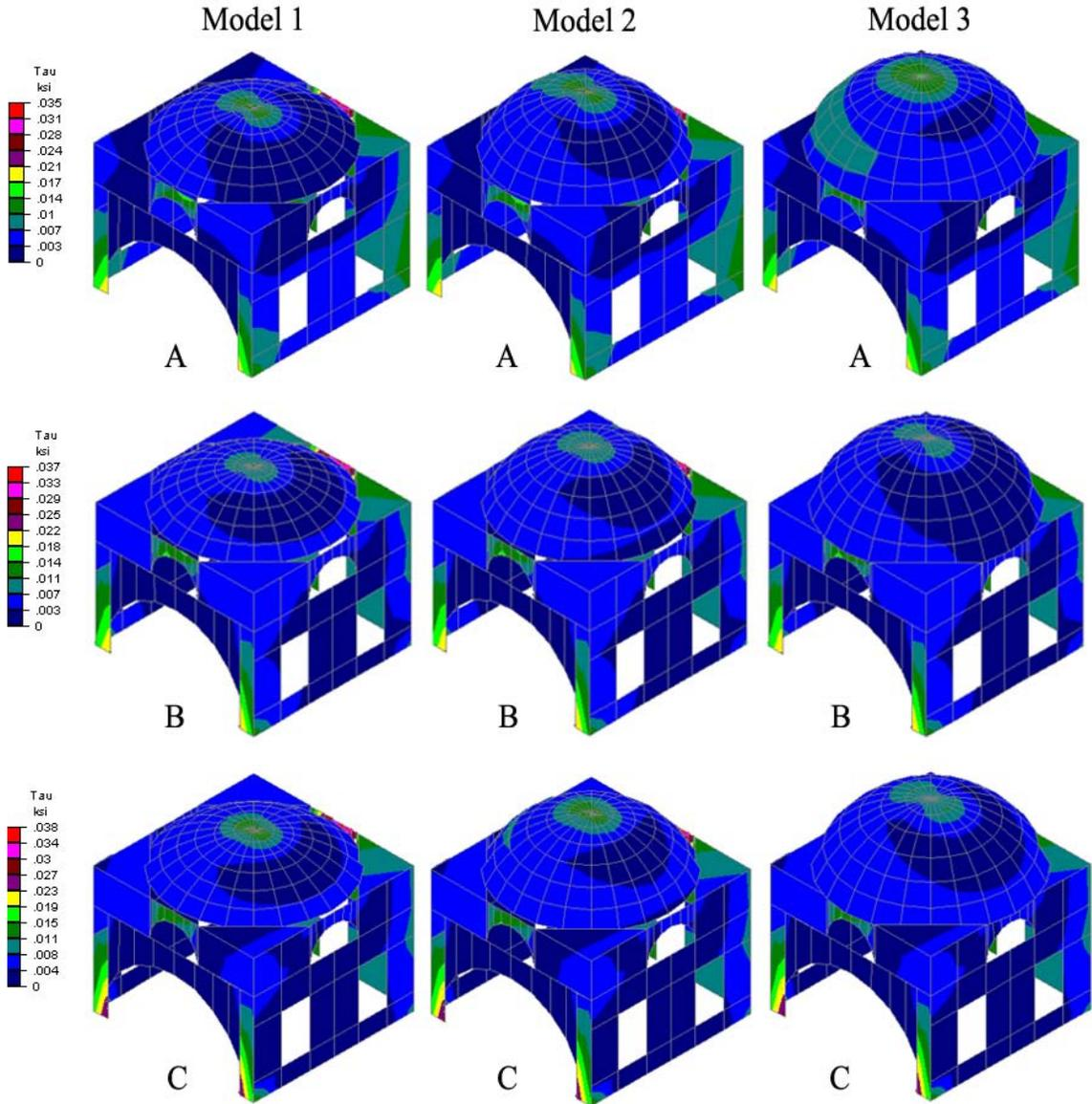
The simulations above show no failure in terms of shear stresses. Highest numbers are half the allowable stresses. The roof domes have little difference in comparison to each other.
