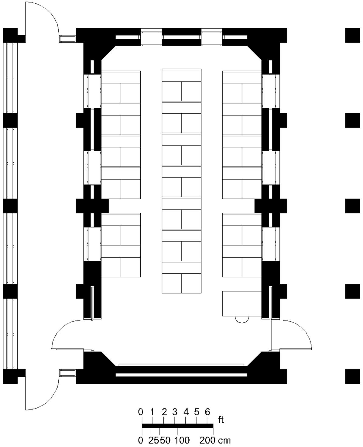
This prototype is divided in three sections: enclosed sunspace or main entry, main classroom unit, and shaded arcade. The clear span of the classroom area is 4.5 meter by 9 meters. It is covered by two domes, which are 4.5 meters by 4.5 meters. The two other areas are covered by a vault type roof. The total unit is a square, 10 meters wide and long. The walls of the main classroom space are 50 cm wide with 10 cm of an air gap.
