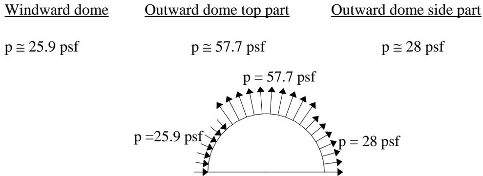
**FIG. 91** WIND LOAD ACCORDING TO THE SHAPE OF THE DOME
