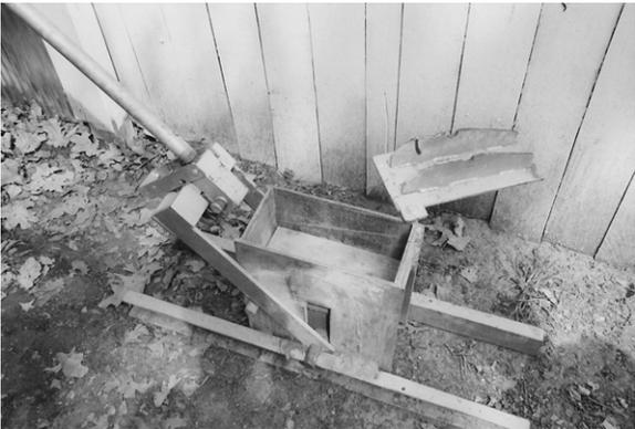
**FIG. 23 STATICALLY COMPACTED MOULD**
