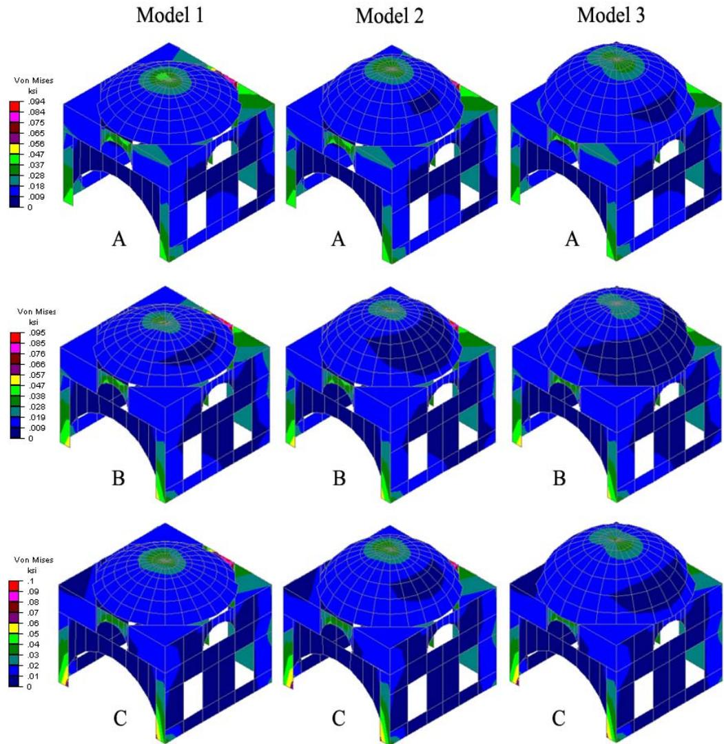
The principal stresses are again lower than the lowest maximum allowable stresses. In comparison, the principal stresses in traditional mud brick, are stressed to possible failure. All model 1 roofs show larger stresses than the other models, but the difference is insignificant.
