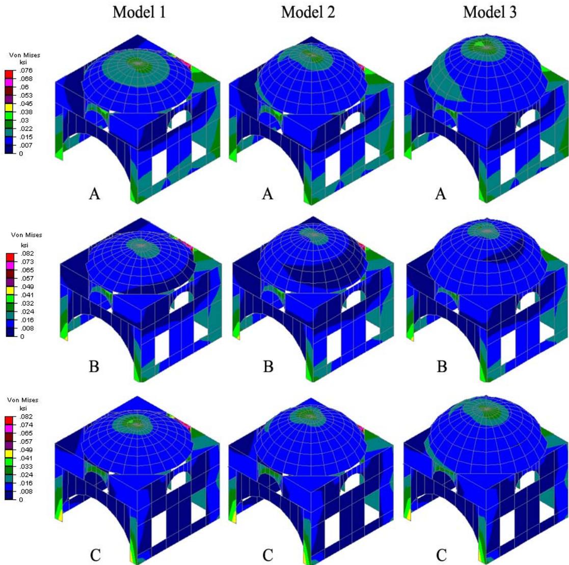
The simulations above show that the stresses are slightly over the allowable stresses that are given on page 102. A simulation with an 80 cm wall gave a better performance for the principal stresses. Under the condition of the maximum (principal) stresses the conclusion can be made that for the resistance of the maximum stresses traditional mud brick construction requires thicker wall sections than 60 cm (24 inch).
