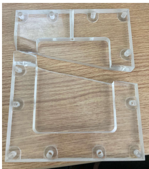
Figure 3: a) Cracked cathode compartment, b) Overall flat-plate MEC with modified polycarbonate cathode compartment installed (right)
