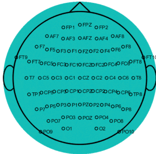
Figure 3.3: Electrode placements for the International 10-20 system
