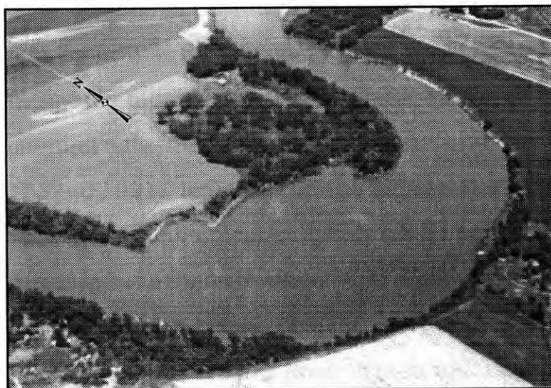
FIGURE 65. The southern meander, pictured here, has not significantly recovered from the channel shape which was present during dredging activities. ( Photo by: Author 1991 )
