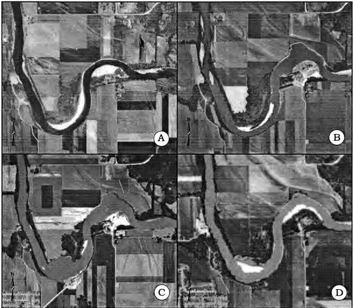
FIGURE 63. Complex channel adjustment in response to sand dredging activities on the lower Big Blue River. A) 1962; B) 1969; C) 1973; D) 1989. (Photo Sources: DOT 1962; ASCS 1969; DOT 1973; NASAAM 1989)
