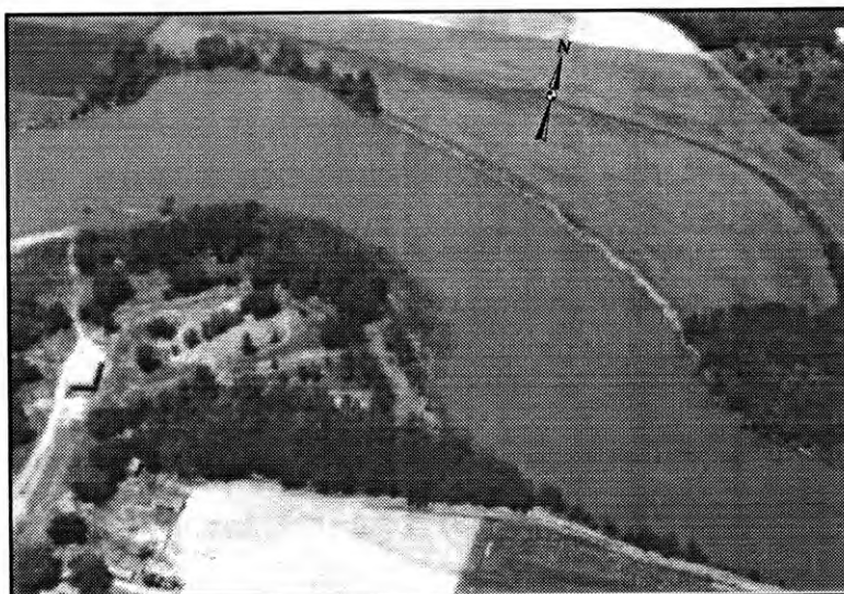
FIGURE 64. The northern channel meander, pictured here, reflects the highest degree of channel healing once dredging activities ceased on the lower Big Blue River. ( Photo by: Author 1991 )
