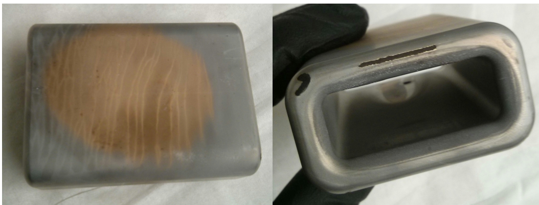
Figure 5.8: Heavily used, TaC-coated graphite susceptors are shown. In the left image, cracks in the TaC coating are visible. In the right image, exposed graphite can be seen after the TaC-coating has flaked off on the top left corner and the top edge.
