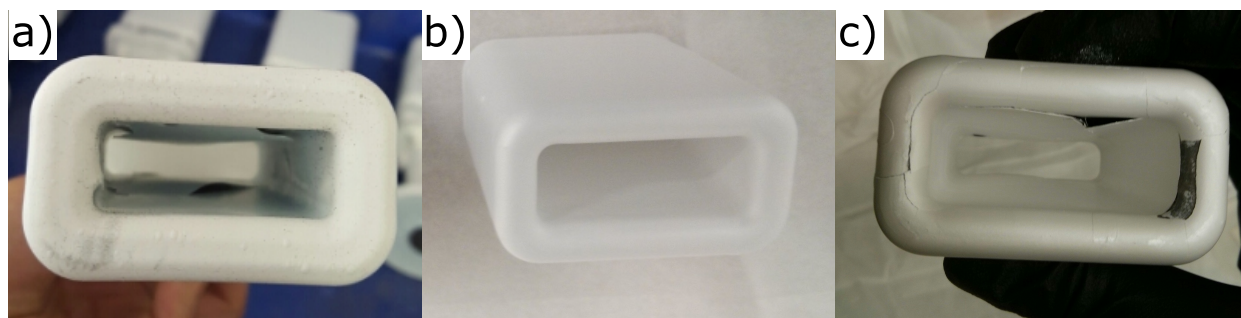
Figure 5.11: a) a graphite susceptor coated with pyrolytic boron nitride. A boron nitride-painted graphite susceptor is shown b) before and v) after heating. The pyrolytic boron nitride film buckles and delaminates from the graphite on the inside of the susceptor. After heating, the boron nitride paint also buckles and delaminated on the interior of the susceptor.
