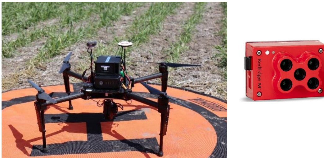
Figure 3.4 The UAV and the camera used for aerial imagery acquisition
