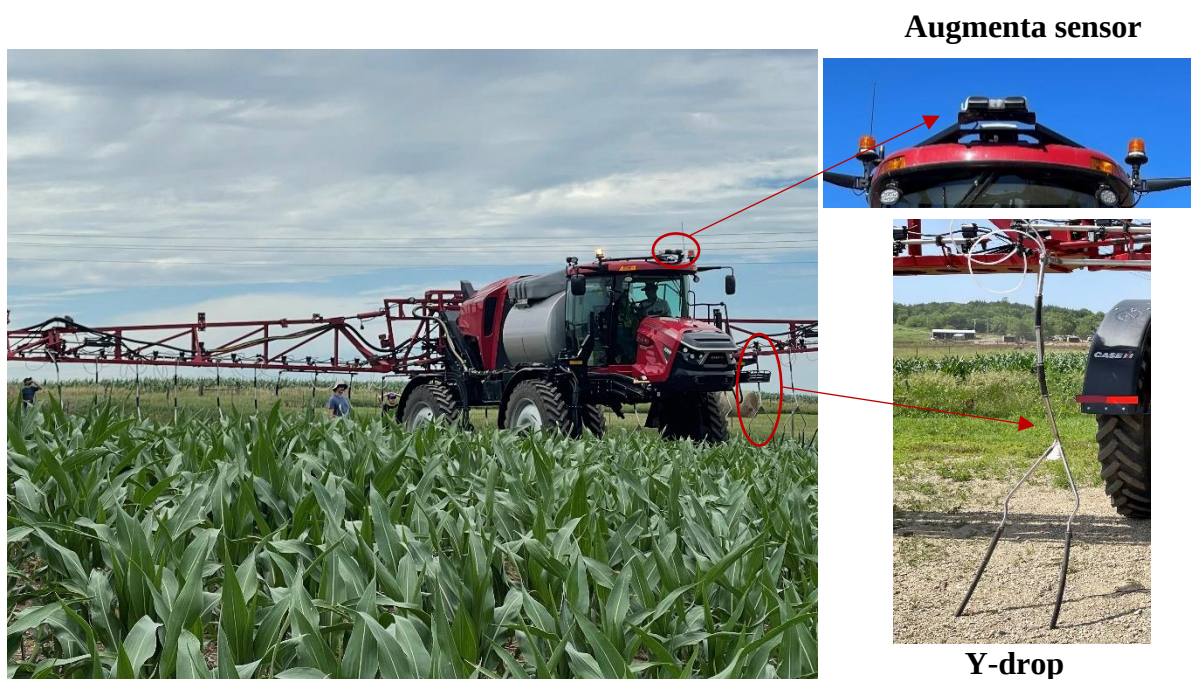
Figure 3.2 Augmenta sensor and Y-drops mounted on the PWM system
