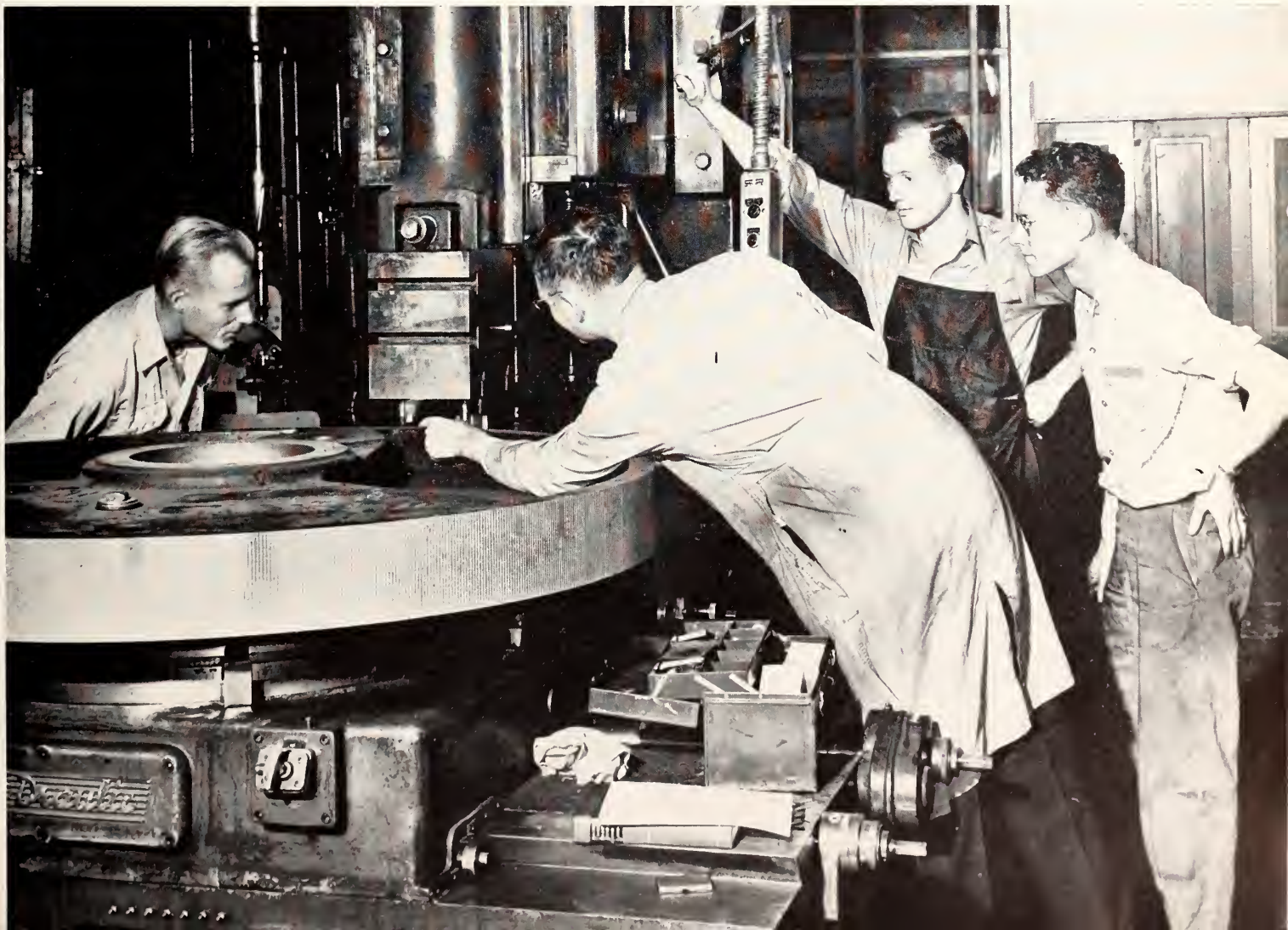
MAKING PARTS FOR A WATCH, NO DOUBT. INSTRUCTOR GIVES A FEW POINTERS IN USE OF BORING MILL TO ENGINEERING STUDENTS.
