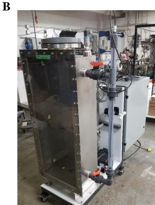
**Figure 7.1** A schematic of the lab-scale gas-sparged AnMBR used in this study (A) and a picture of the system (B).
