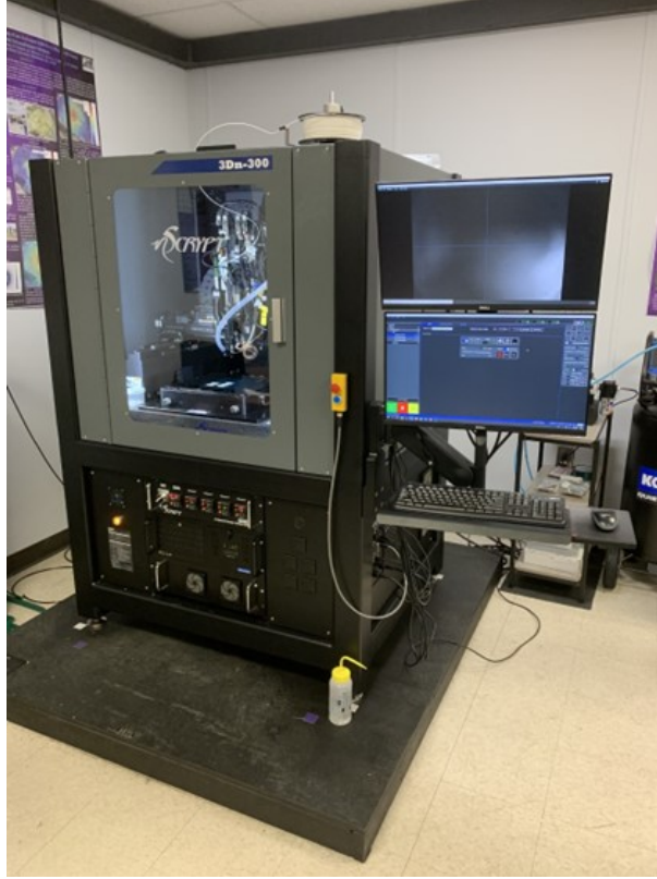
Figure 3.1: The 3Dn-300 multi-functional 3D printer with enclosed build plate.
