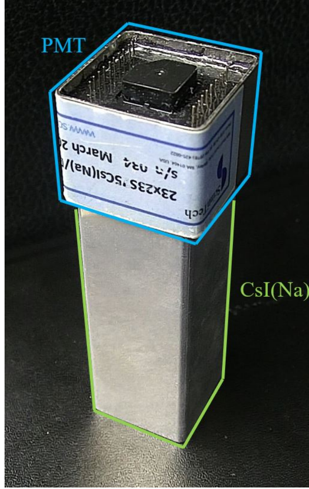
Figure 2.1: The R11265U PMT and CsI(Na) crystal assembly.
