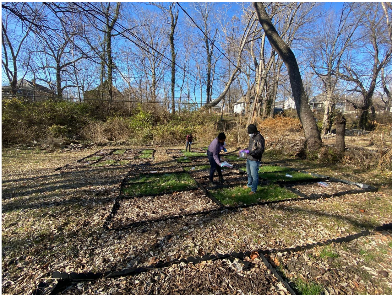
Field soil sampling using a manual soil probe within established experimental plots.
