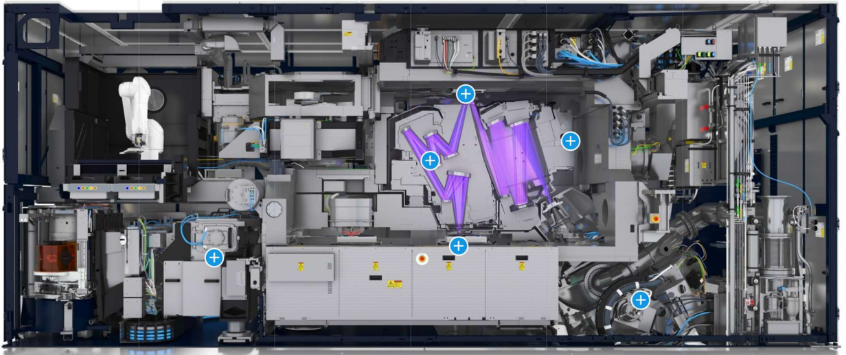
Figure 7: Inside of NXE lithography system [7]
