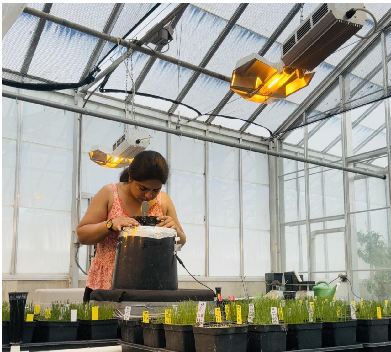
Figure C.4. Digital image collection for turfgrass cover assessment (percent green cover) using digital camera.
