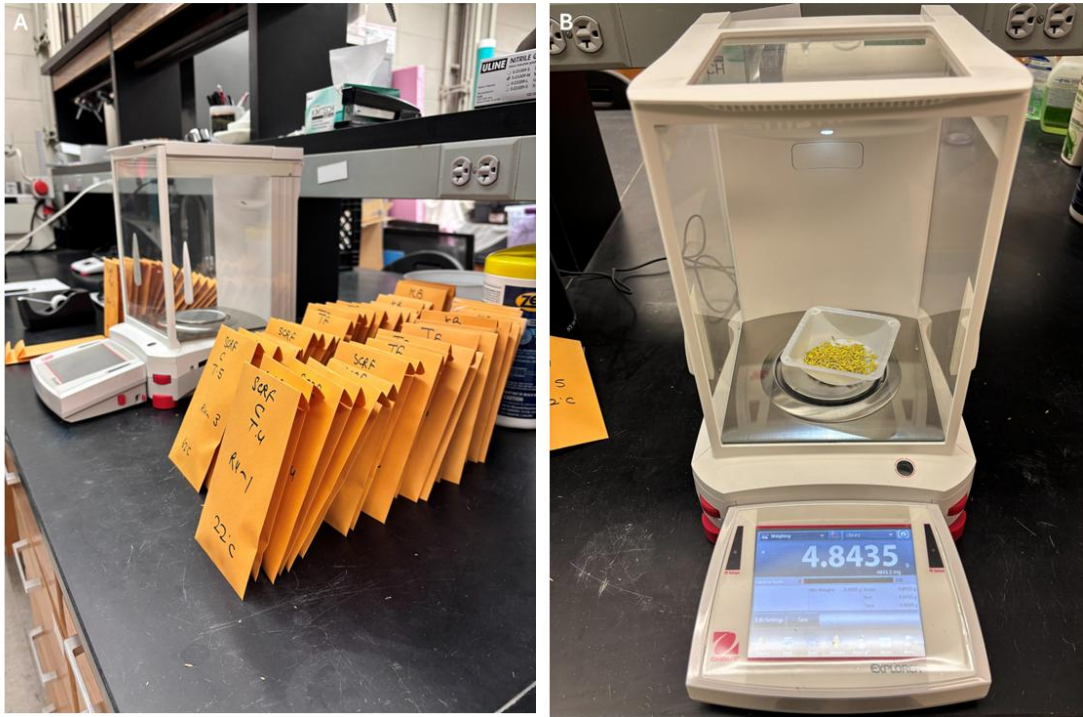
Figure B.1. Seed sample preparation and weighing for seed moisture content determination. (A) Labeled seed envelopes organized prior to weighing. (B) Coated turfgrass seed weighed using an analytical balance before seed moisture content analysis.
