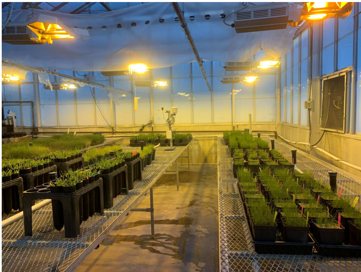
Figure C.1. Greenhouse experimental setup for evaluating seed coating, irrigation regime, and soil type effects on turfgrass establishment at the Throckmorton Plant Science Center greenhouses, Kansas State University.
