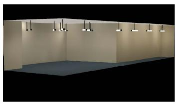
Figure 6-3: AGI32 rendering of suspended indirect/direct fixture layout for a typical classroom.
