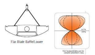
Figure 3-2: Direct/indirect suspended fixture cross section and light distribution illustration
