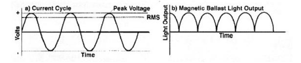
Figure 2-2: Sinusoidal graph comparing the frequency of current to perceived cycle of light Shown is the operation of a magnetic ballast, which is the most noticeable, but the graphical representation applies to any output of light operating with a ballast (Ryan, Eileen. 2007).
