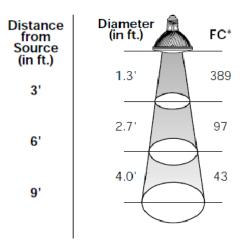
Figure 6-4 Conic distribution of light from a 60W PAR 30 normal flood lamp. (Sylvania, 2010).
