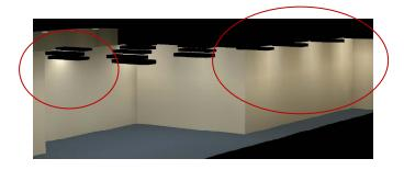
Figure 6-6 Rendering of recessed fluorescent fixtures The image shows the problem glare and hot spots on vertical surfaces.
