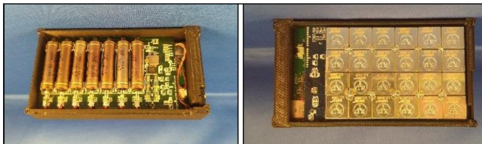
Figure 6-1 The MGDs (Left) & MNDs (Right) communicated with the android application (Top) either through a wired zero-RF low voltage differential signal (LVDS) or wirelessly through a low energy Bluetooth.
