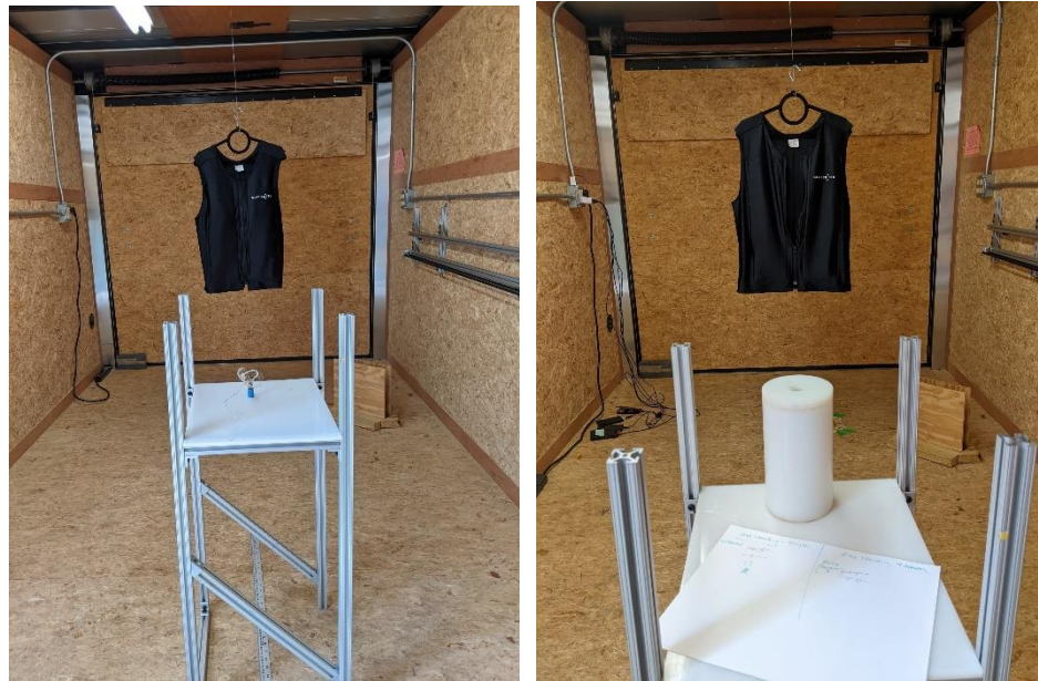
Figure 7-7 The free standing ARGANOT system is pictured. The vest was populated with up to eight modules and exposed to a bare and moderated ^{252}\text{Cf} source.
