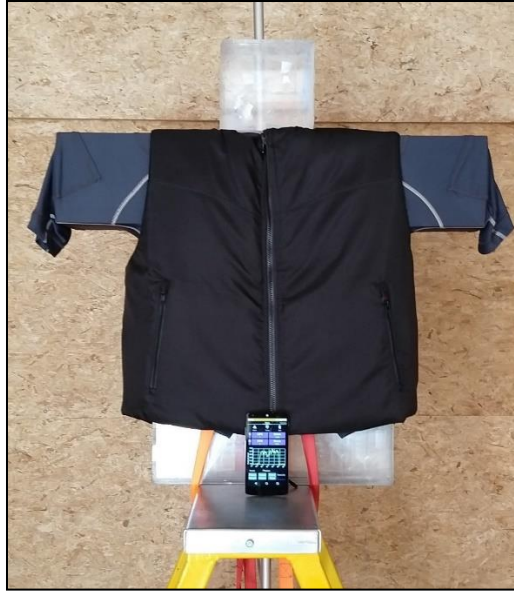
Figure 6-3 16 MND modules and 2 MGD modules were discretely implanted into the vest worn by the phantom. All data was fed to the users lifetime via the android cell phone.
