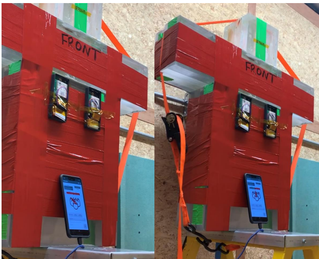
Figure 7-48 Two of the four ARGANOT modules distributed across the phantom's body are shown communicating livetime directionality information to the android advice. As shown on the left, the source is initially located to the left of the phantom. As the source approaches the phantom, the android device alerts the user that the source is in front of them.
