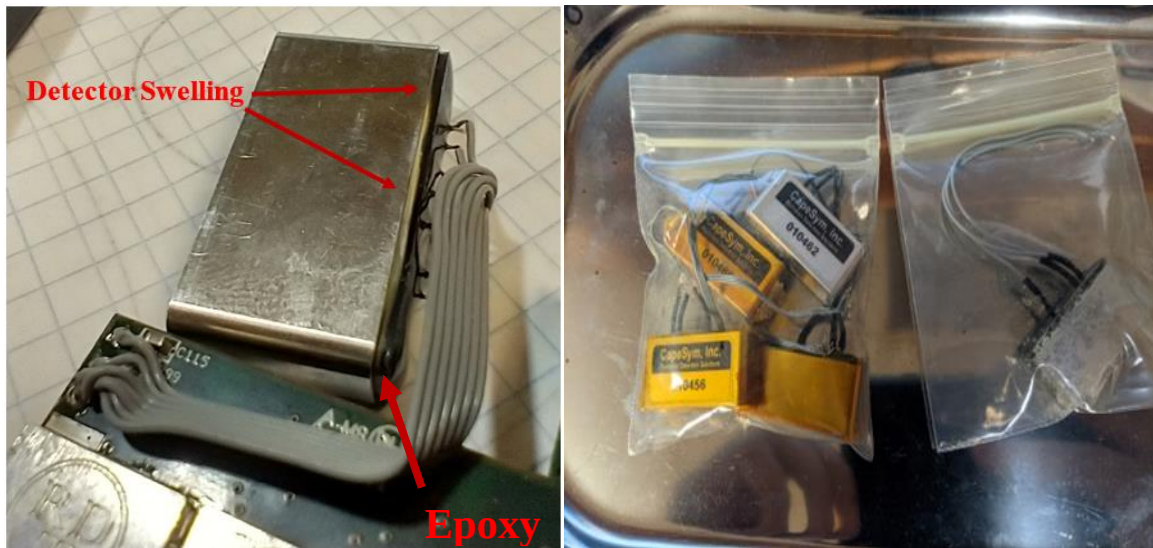
Figure 5-19 Several detectors swelled and often leaked yellow fluid. When detectors were identified to have a faulty hermetic seal, the detector was isolated and properly disposed of.
