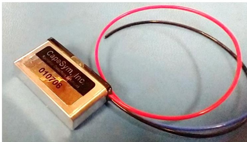
Figure 5-23 Version four of the Capesym SrI 2 gamma-ray detector with light-tight lid and relocated wire output.
