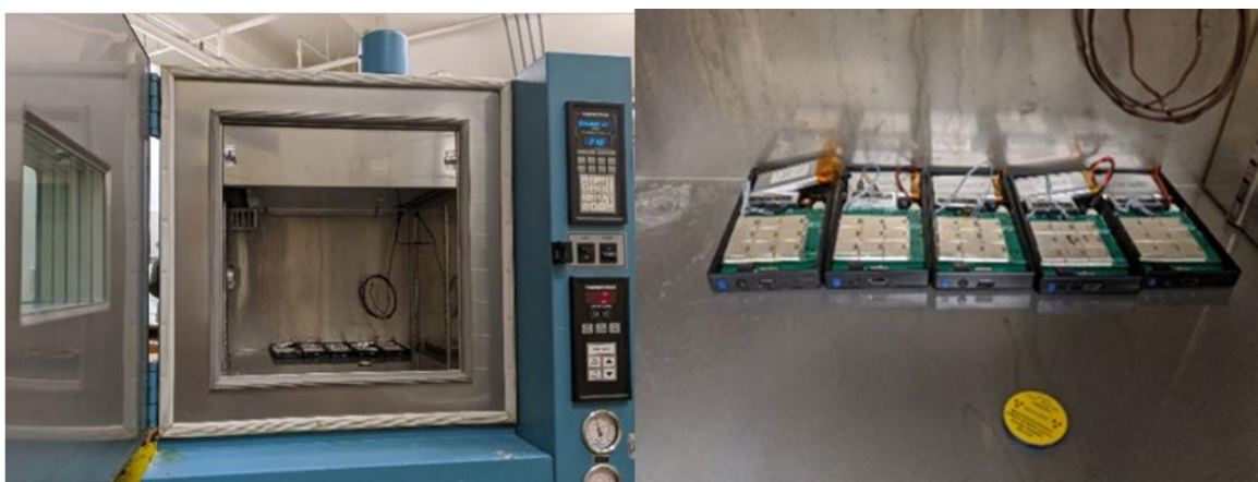
Figure 5-28 The module devices were placed in a temperature and humidity-controlled chamber to maintain a stable environment for testing and calibration. A 137 Cs source is shown above in front of five of the ARGANOT modules while conducting a mission (right).
