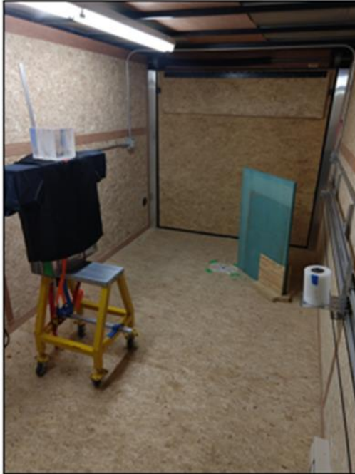
Figure 7-31 The phantom is shown wearing the ARGANOT populated garment as the moderated ^{252}\text{Cf} neutron source passes on the mail.
