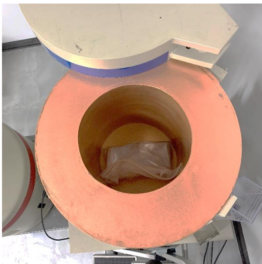
Figure 3-4 The suspected contaminated Pb brick was place over top of the HPGe detector head and a long measurement was conducted.
