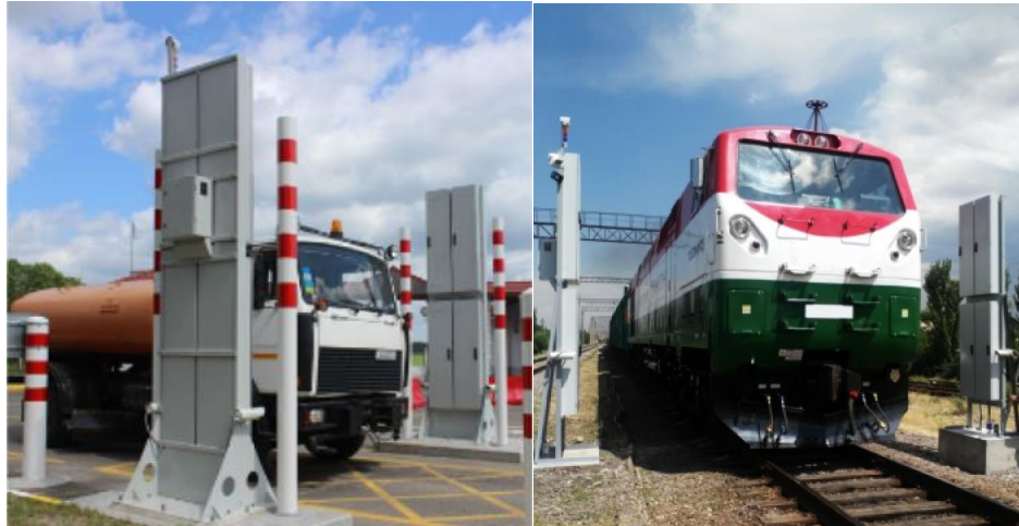
Figure 2-1 An example passive radiation monitor is shown alongside of a railroad [10].
