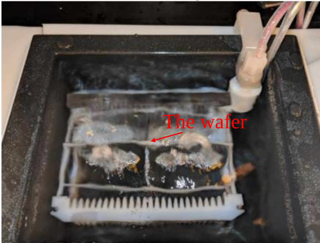
Figure 4-16 The mega sonic tank in operation with the wafer placed into the wafer boat is shown.
