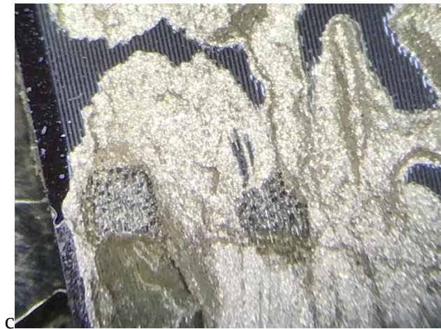
Figure 4-30 The silver epoxy used to adhere the device to the PCB was found to leak into the trenches. Upon heating, the epoxy would cure and expand within the trenches of the devices, increasing the leakage current.
