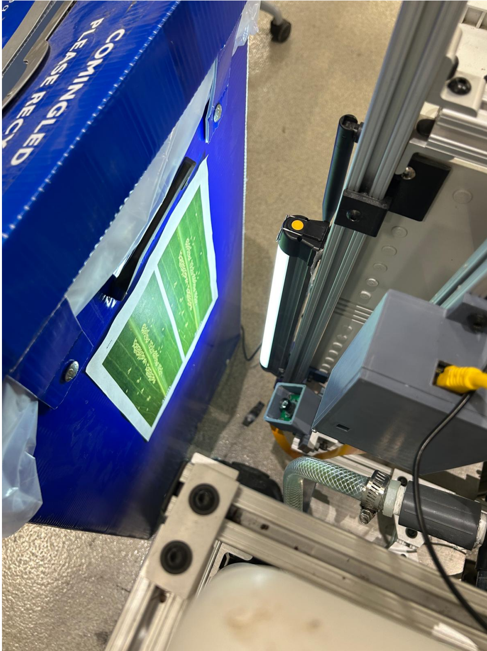
Figure 3.19: External view of the experimental setup with the camera at a 40-degree upward angle.
