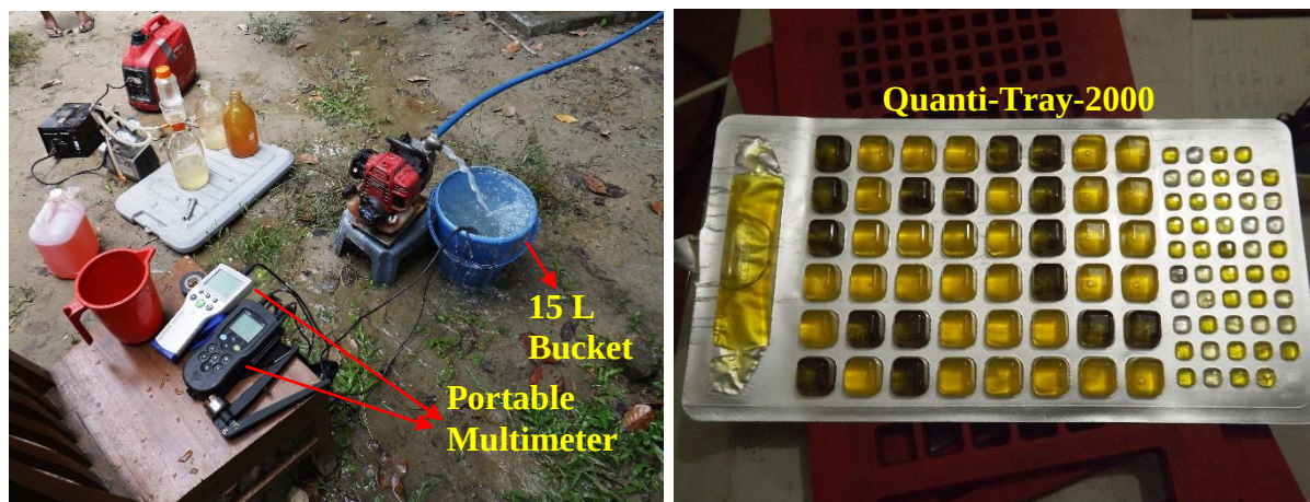
Figure 5.4 On site parameter measurement and MPN based Colilert test
