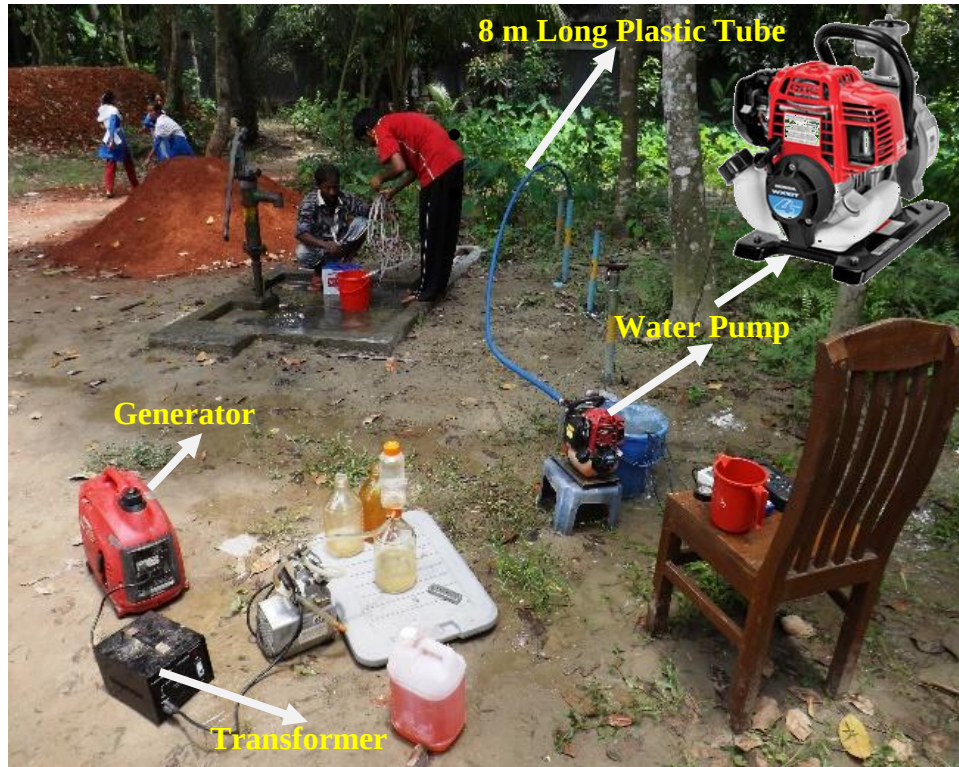
Figure 5.3 Process showing cleaning of water pump and filtering water sample in field
