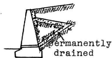
(g). Expansive Backfill
