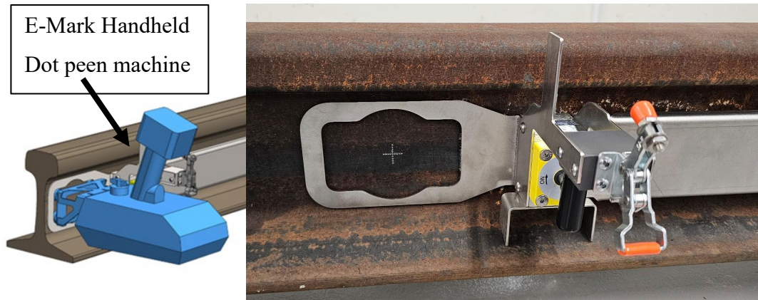
Figure 3.17 Dot-Peen Marking Using Magnetic Template
