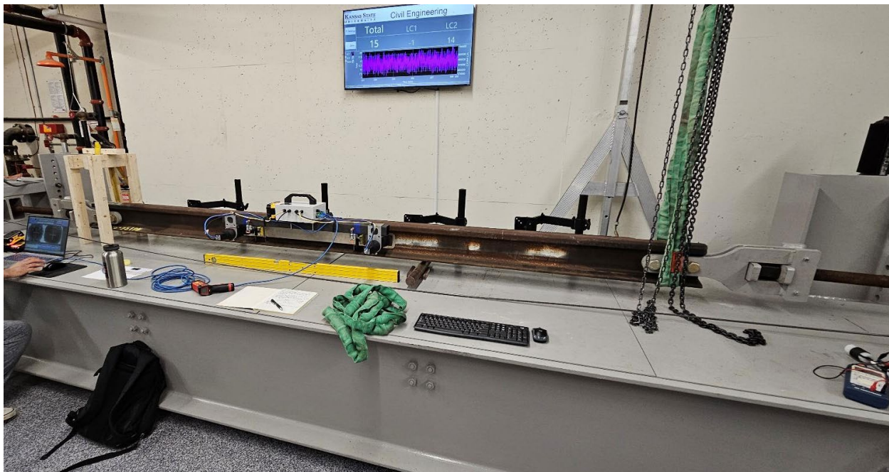
Figure 8.1 Long Rail Section Installed on Testbed
