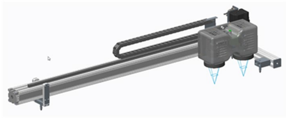
Figure 3.1 Automated Dual-Camera System [8]
