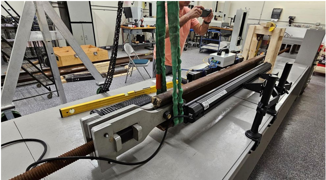
Figure 8.3 Short Rail (77") Section on Testbed with IR Heater Installed
