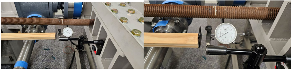
Figure C.3 Dial Gage Connection with Wooden Stick for Deflection Measurement
