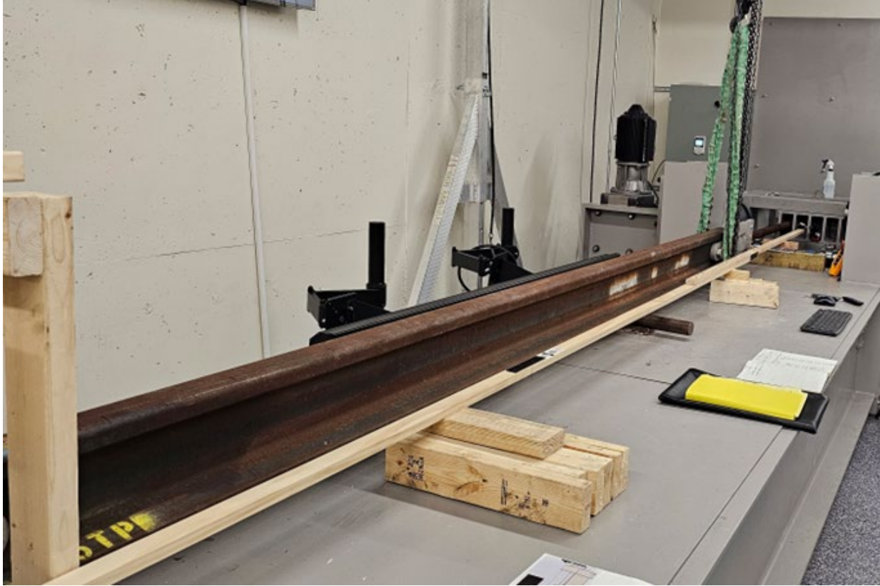
Figure C.1 Wooden Stick Connected to Testbed on One End and a Dial Gage on the Other
