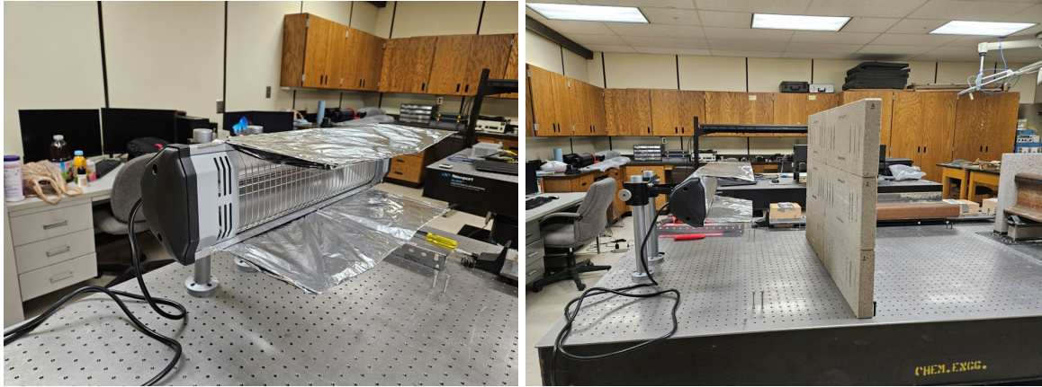
Figure G.5 Commercial Heater with Aluminum Blades for Radiation Convergence
