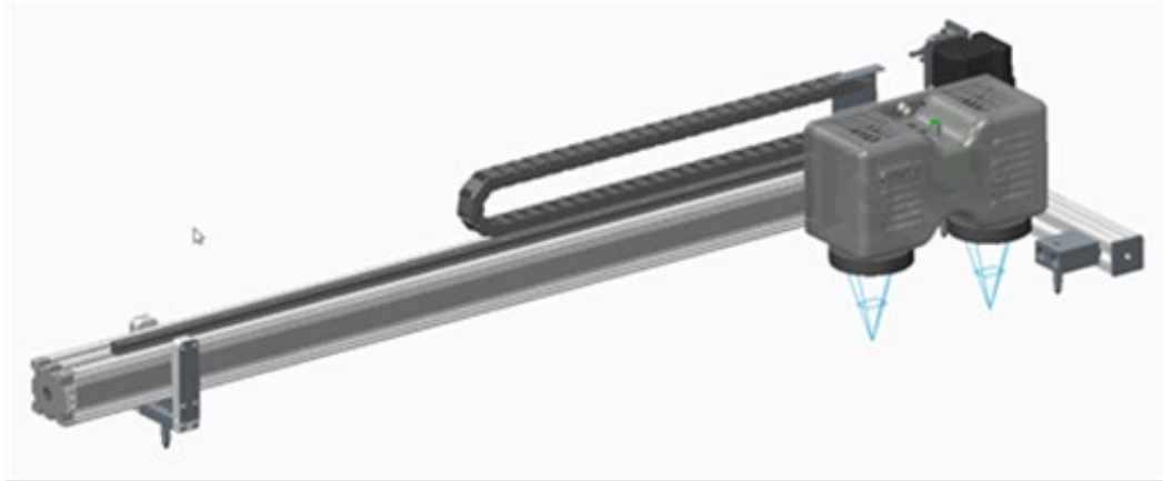
Figure 2.3 Automated Dual-Camera System [8]
