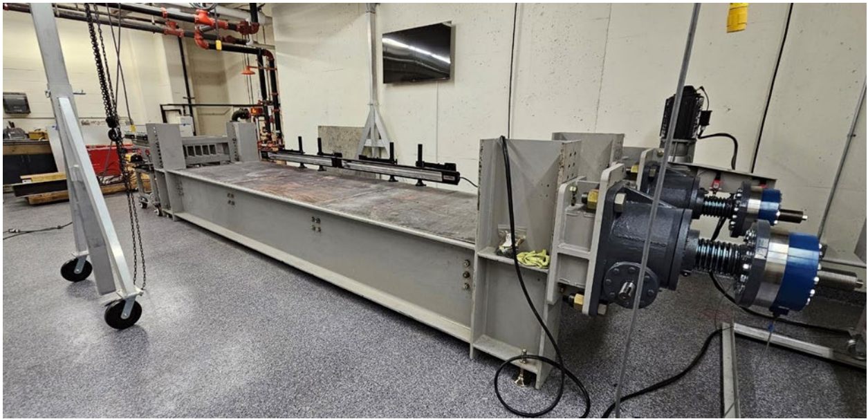
Figure 8.2 IR Heaters Installed on Testbed for Controlled Thermal Heating
