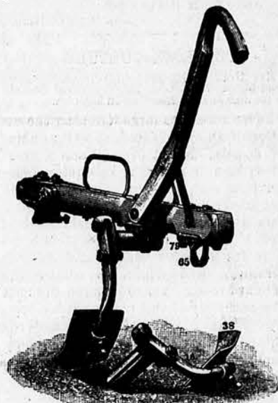
Adjustable standard casting, showing construction used on No. 2 Hamilton Cultivator.
