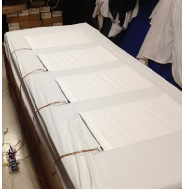
Figure 2.2: Designed bed system with four film sensors (EMFi's).
