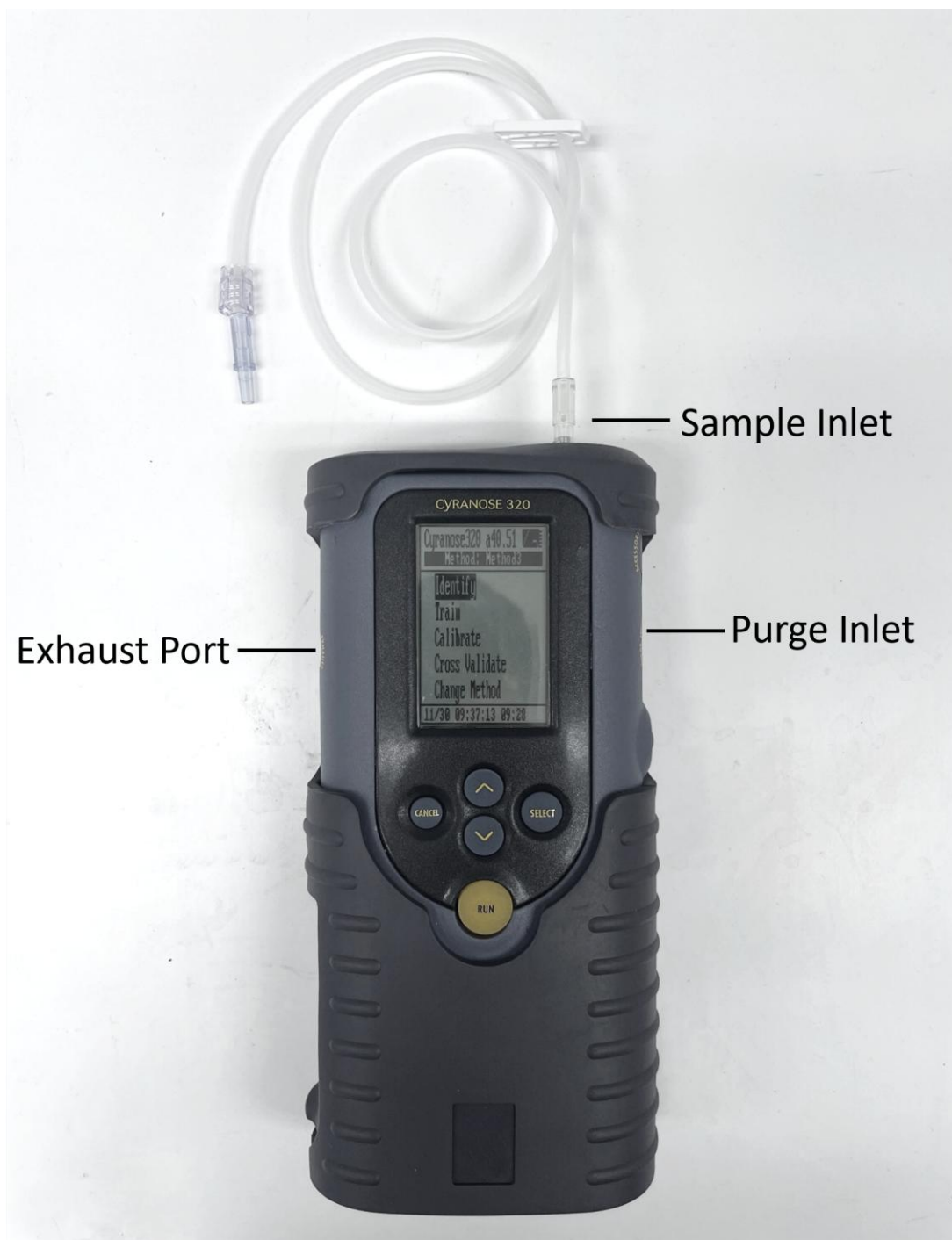
Figure 6.1. Cyranose 320®* eNose with labeled features.
