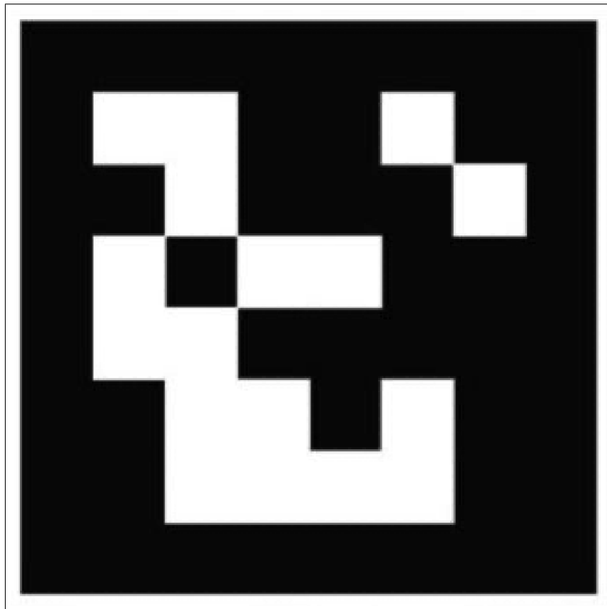
Figure 3.7: Aruco Marker with 6x6 dictionary and Id no 3.
