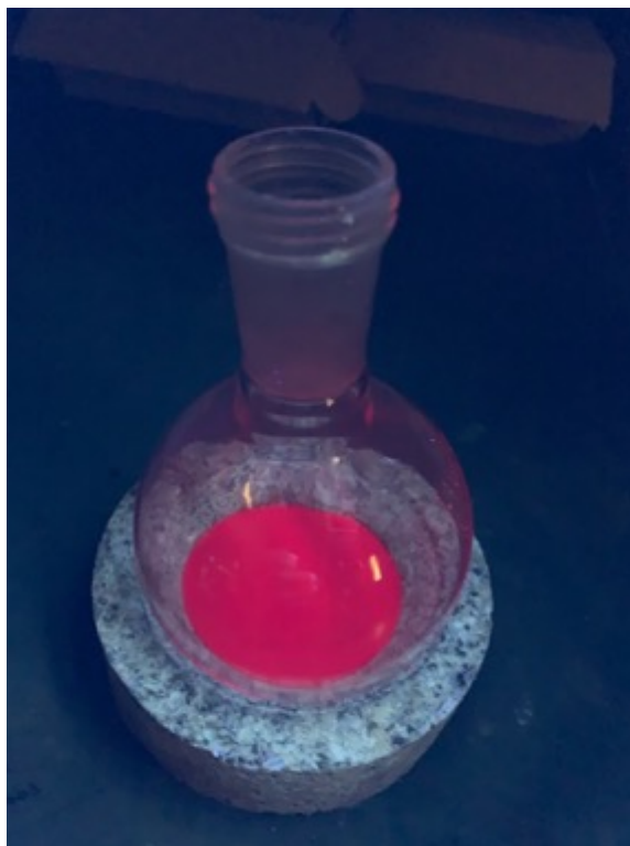
Figure 59: TCP in methanol under UV lamp (365nm)
