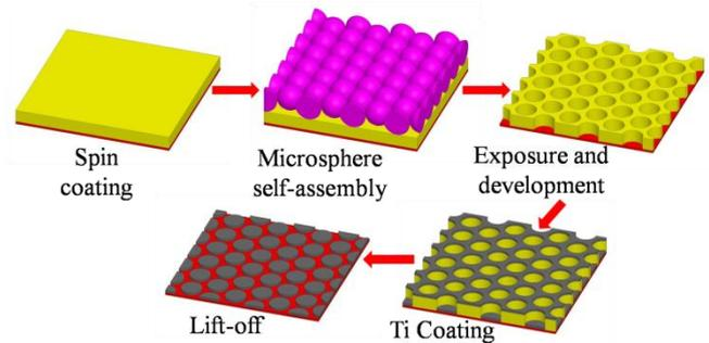
Figure 1. Schematic of Ti nanopillar fabrication process
