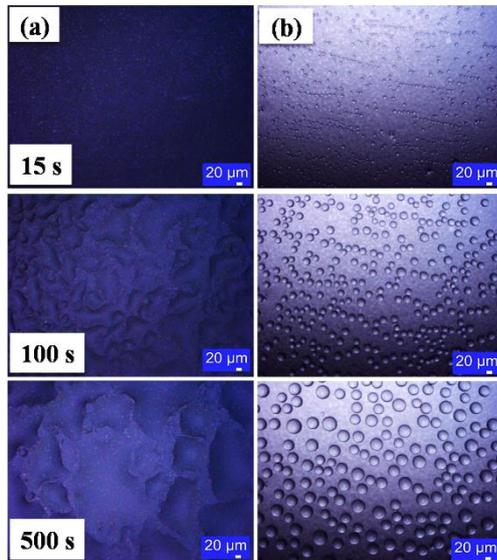
**Figure 5.** Time-lapsed droplet growth on (a) plain Ti pillared (b) Teflon® coated hydrophobic Ti pillared glass surfaces at  $35 \pm 5\%$  RH and  $275 \pm 0.2\text{K}$  surface temperature.
