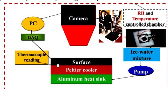
Figure 3. Schematic diagram of the experimental setup in a RH controlled chamber
