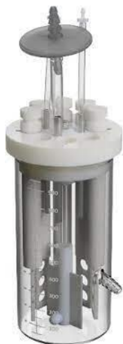
Figure 1.1 CDC Biofilm Reactor from Biosurface Technologies Corporation (Bozeman, MT).
