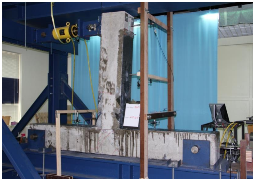
Figure 2.1. The Experimental Failure of The One of The Four Specimens Occurring at The Column Critical Region (Saqan et al. 2020).
