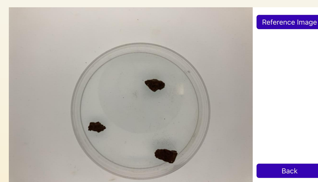
Figure 2: Screen shot of the Slakes app, with the camera pointed at three dry soil aggregates placed in a petri dish.
