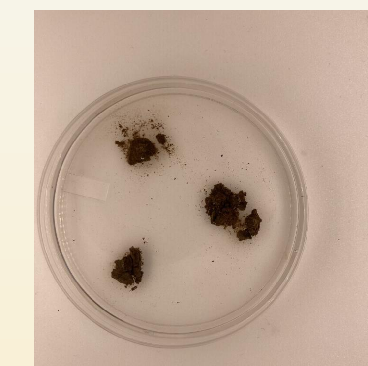
Figure 5: Three aggregates after they have been soaking in water.
