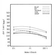
Figure 6. DSC Endotherms of Wheat Starch at 3 Water:Starch Ratios (2:1, 1:1 and 0.5:1).
