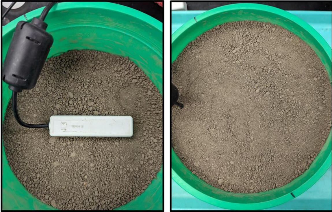
Appendix A Figure A- 2 Calibration of TEROS 12 with dry ( 0 \text{ cm}^3 \text{ cm}^{-3} ) silty clay loam soil in a bucket of 4,000 \text{ cm}^3 .
