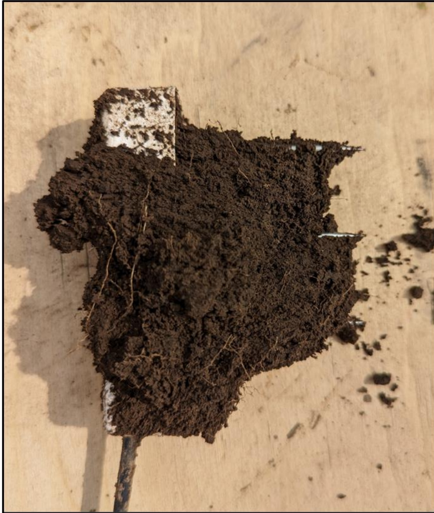
Appendix B Figure B- 4 TEROS 12 soil moisture sensor placed outside the instrumented microlysimeter within the row crop, with surface roots surrounding the sensor rods.
