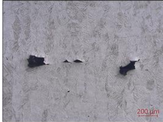
Figure 1.3. Example of LOF porosity in L-PBF Ti alloy. (Included with permission from Elsevier) [33].
