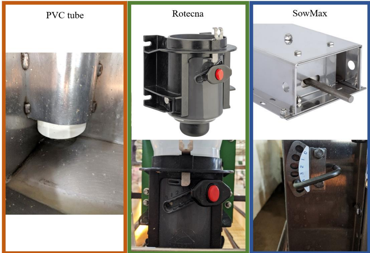
Figure 5.2. Sow lactation feeders, feeder trigger, and adjustment mechanisms.
