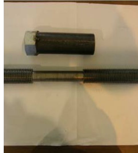
Figure 10: Mild Steel Energy Dissipator
