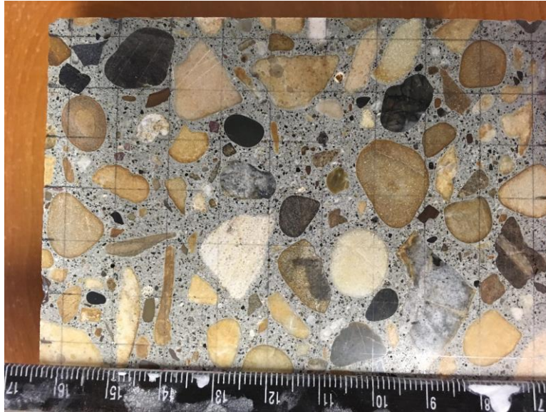
Figure 133. Polished samples with 1 cm 2 grids for DRI method
