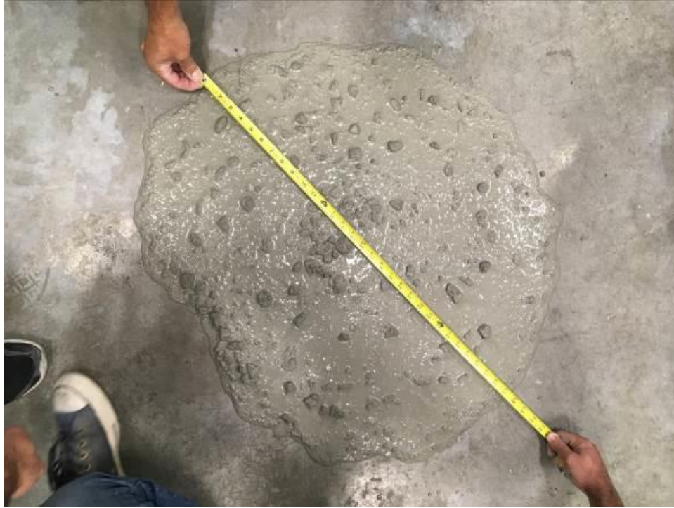
Figure 63. Slump-flow (spread) of segregated mix (B161)
