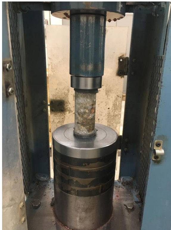
Figure 102. Compressive strength test setup for 2 in. diameter cores
