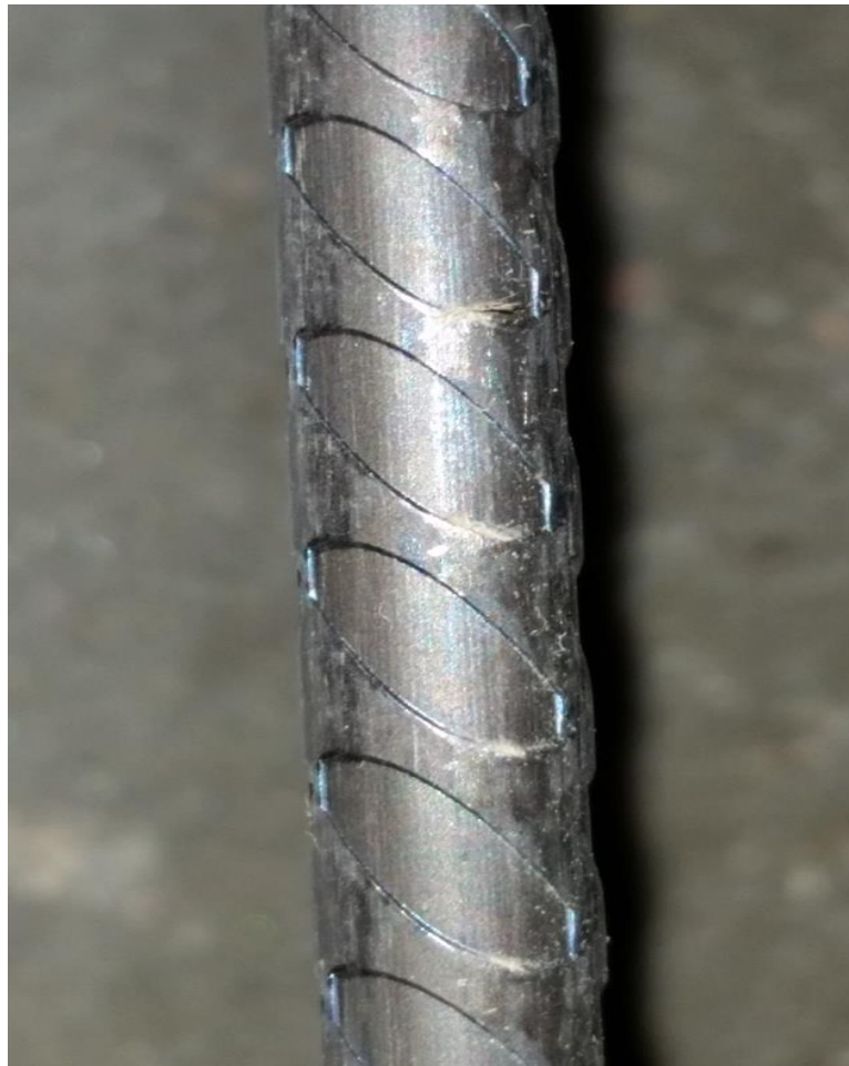
Figure 55. Close-up view of indentation pattern of WP wire
