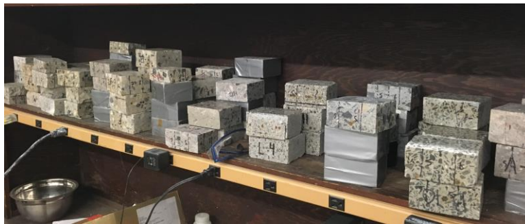
Figure 100. Sliced samples from 12 different types of ties
