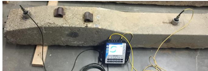
Figure 138. UPV transducers on good tie in mid to shoulder position
