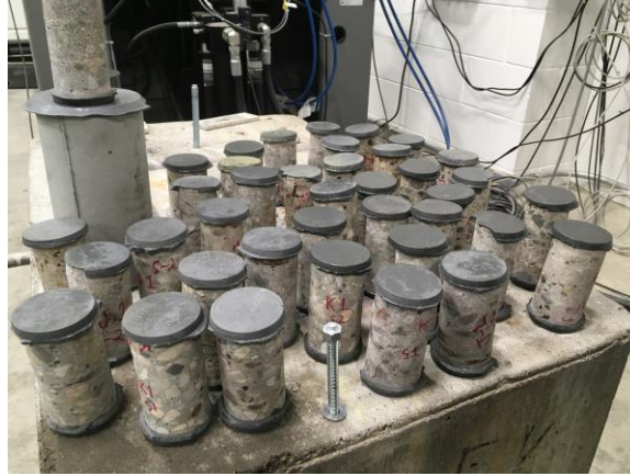
Figure 101. Capped cores extracted from the ties
