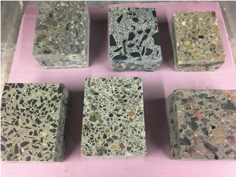
Figure 108. Polished samples from 12 types of ties
