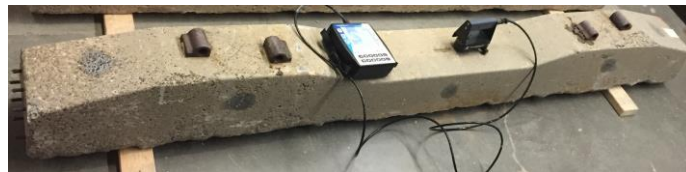
Figure 145. IE device on the middle of one of the uncracked ties
