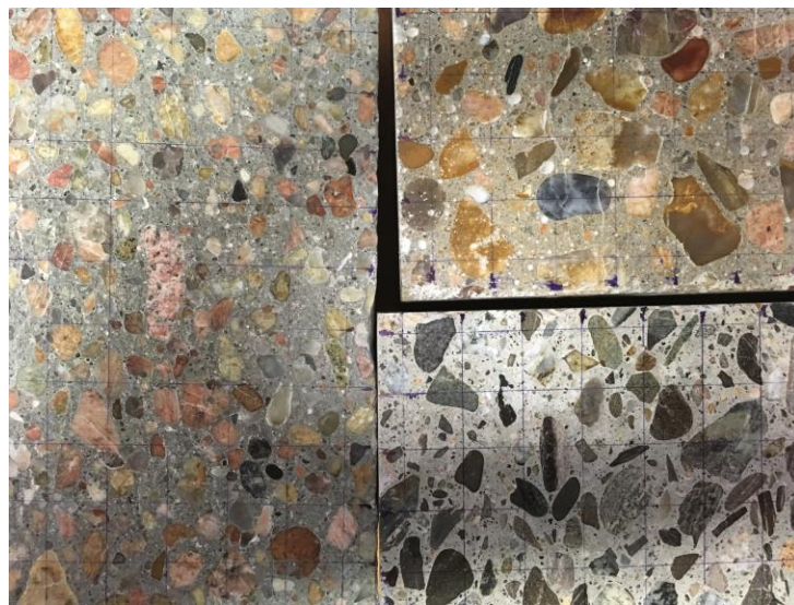
Figure 132. Polished samples for DRI method
