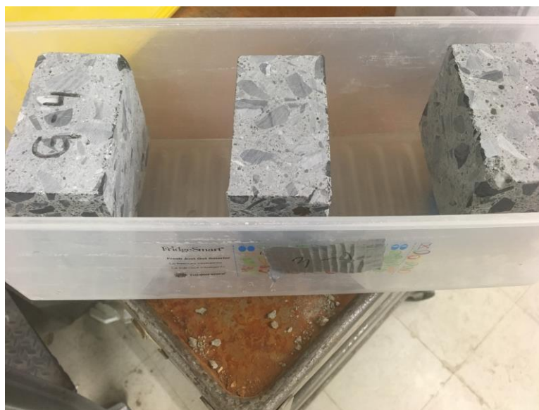
Figure 111. Pre-conditioned samples for absorption test
