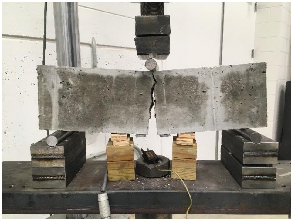
Figure 21. Fatigue crack growth test set up.
