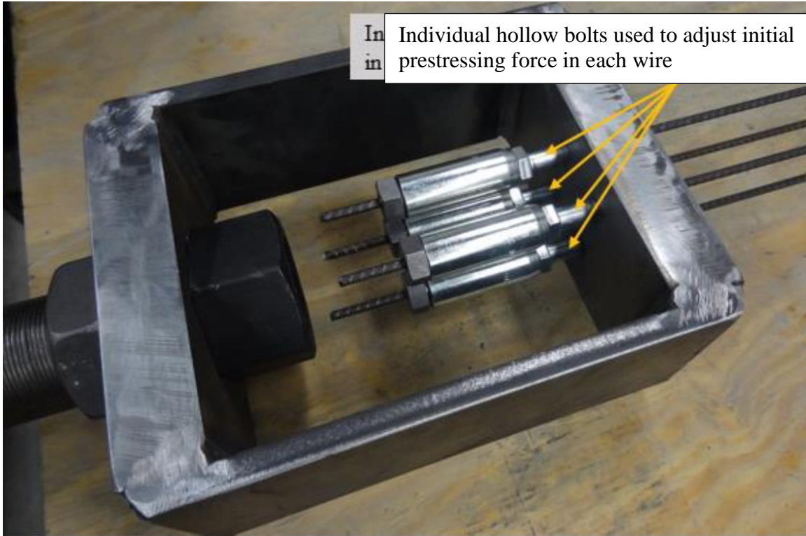
Figure 53. Hollow bolts adjacent to anchor chuck were used to manually adjust the initial prestressing initial force in each wire to 300 lb
