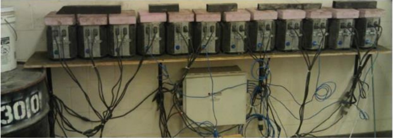
Figure 58. A commercial “Sure-Cure” system was used to temperature-match cure the test cylinders
