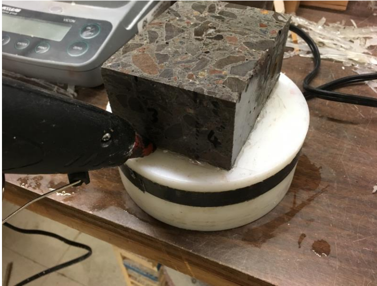
Figure 128. Mounting samples on polymeric cylinder
