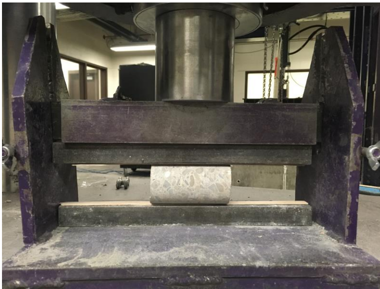
Figure 104. Splitting tensile test setup for 2 in. diameter cores
