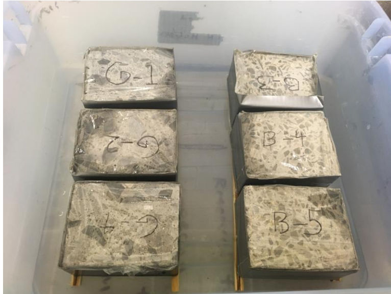
Figure 112. Covered samples placed on water surface
