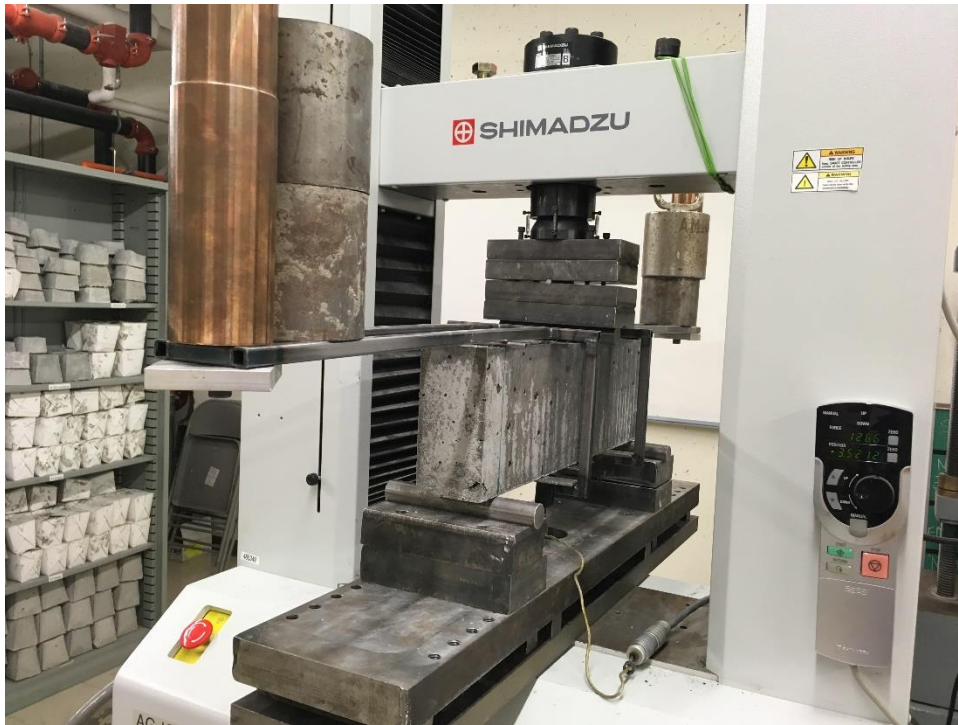
Figure 18. Fracture toughness test setup
