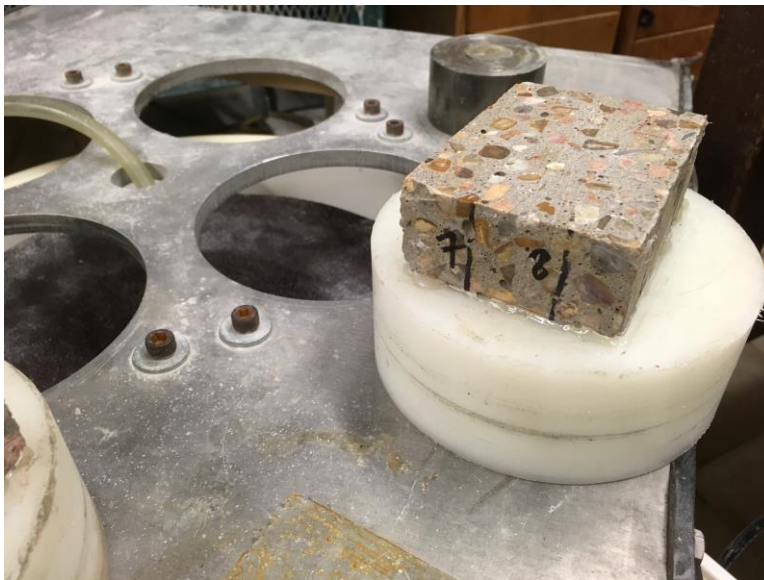
Figure 129. Prepared samples for abrasion test
