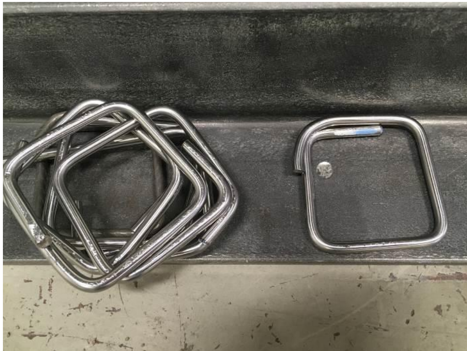
Figure 82. Stirrups with 5 bends made at KSU lab
