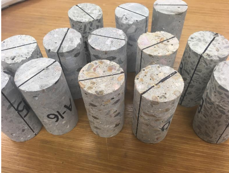
Figure 103. Prepared cores for splitting tensile test
