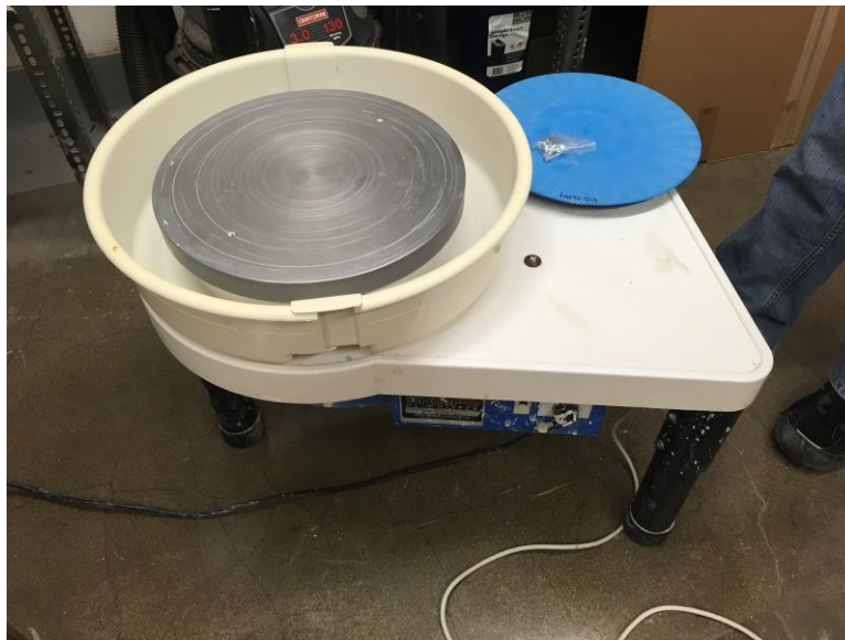
Figure 127. Pottery wheel used for abrasion test
